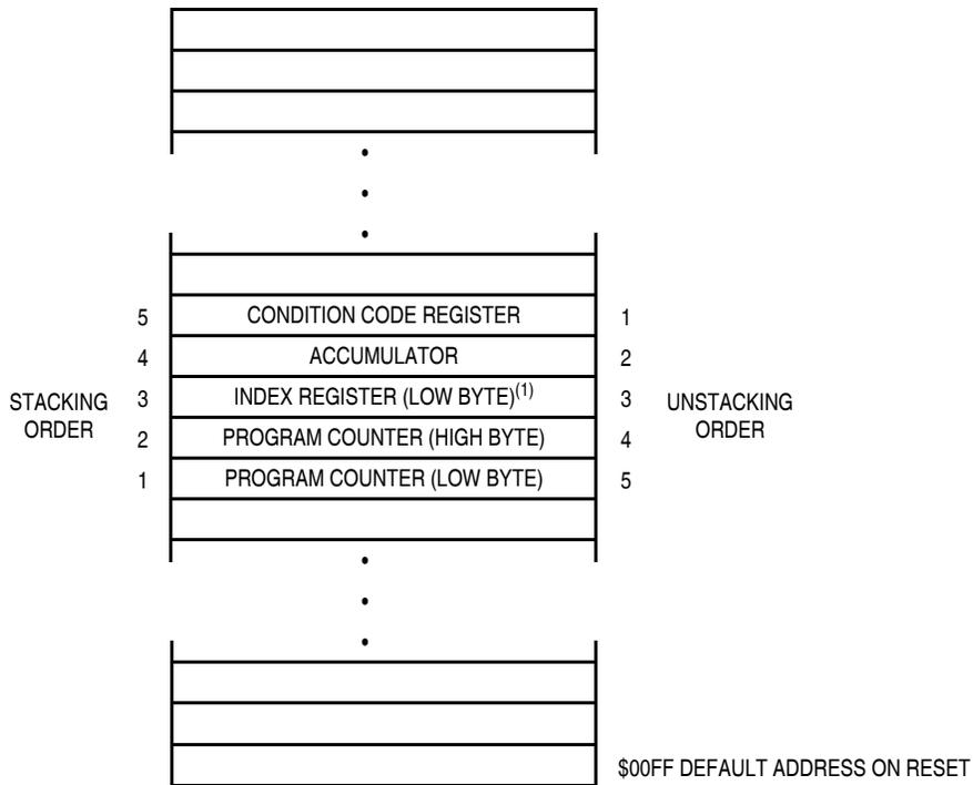
1. High byte of index register is not stacked.
