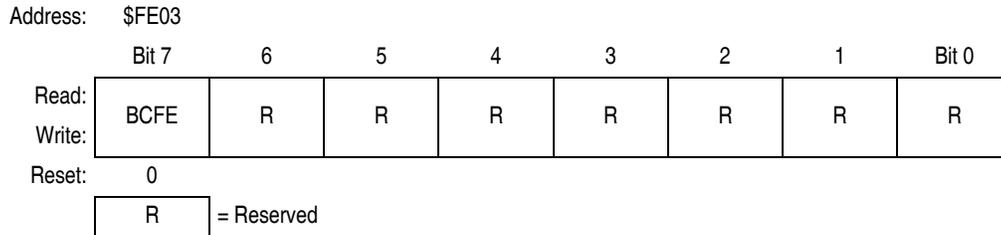
**Figure 15-22. SIM Break Flag Control Register (SBFCR)**
