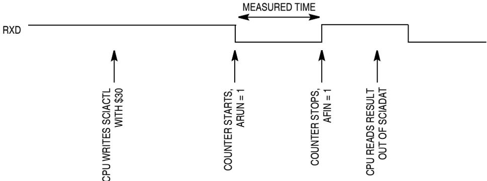
Figure 14-23. Bit Time Measurement with ACLK = 1, Scenario B
