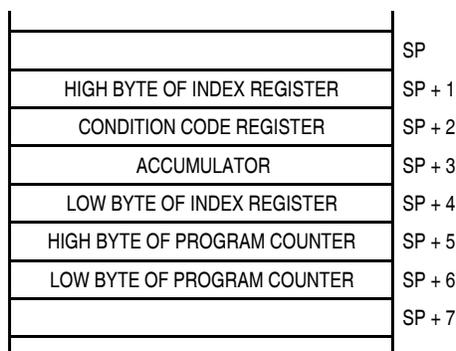
**Figure 19-17. Stack Pointer at Monitor Mode Entry**
