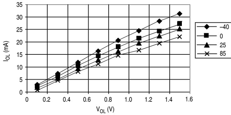
$V_{OL} < 0.4 \text{ V} @ I_{OL} = 1.6 \text{ mA}$
