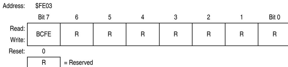
**Figure 19-8. SIM Break Flag Control Register (SBFCR)**
