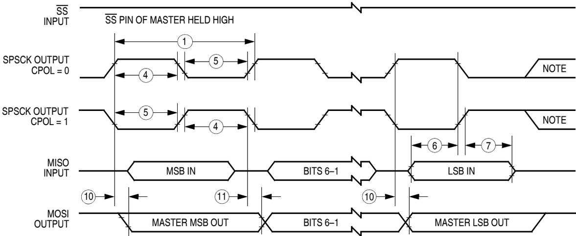
Note: This last clock edge is generated internally, but is not seen at the SPSCK pin.
