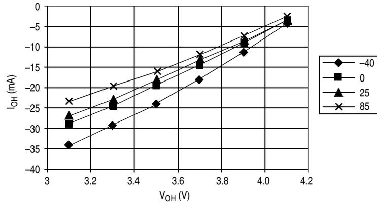
$V_{OH} > V_{DD} - 1.5 \text{ V} @ I_{OH} = -20.0 \text{ mA}$
