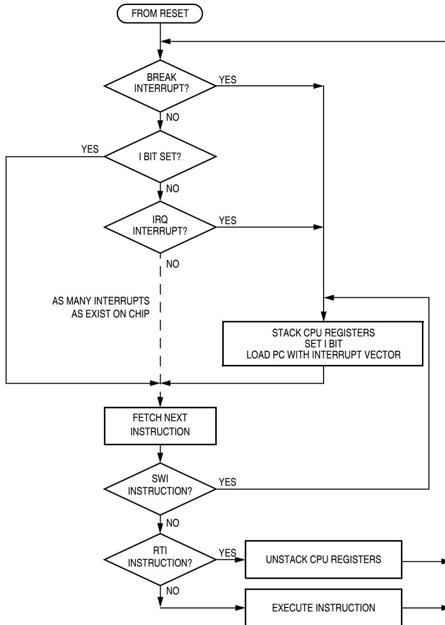
**Figure 15-10. Interrupt Processing**
