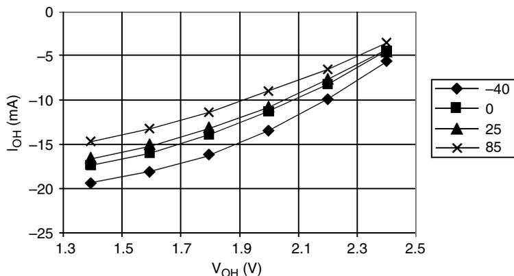
$V_{OH} > V_{DD} - 1.0 \text{ V} @ I_{OH} = -10.0 \text{ mA}$
