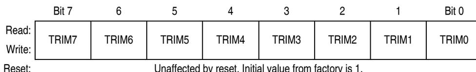
Write to this register is by a programming sequence to the Flash memory.
