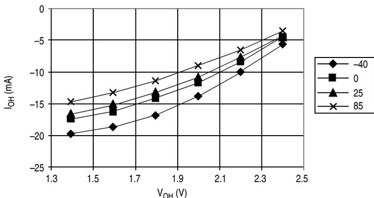
$V_{OH} > V_{DD} - 0.3 \text{ V} @ I_{OH} = -0.6 \text{ mA}$
