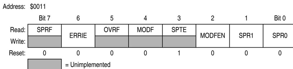
**Figure 16-15. SPI Status and Control Register (SPSCR)**
