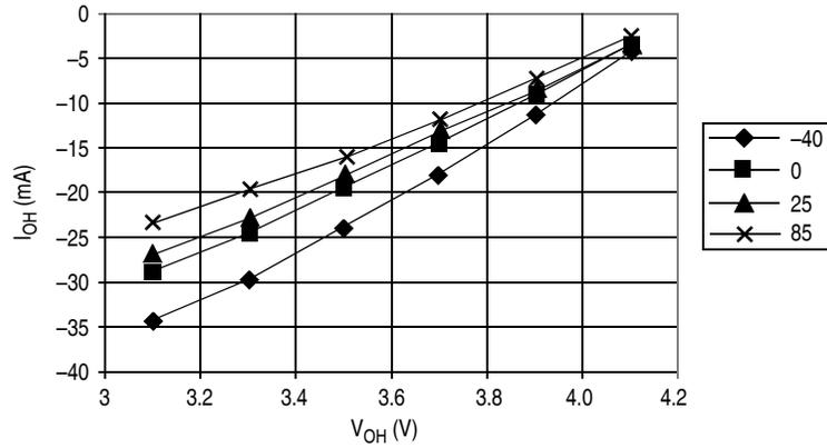
$V_{OH} > V_{DD} - 0.8 \text{ V} @ I_{OH} = -2.0 \text{ mA}$
