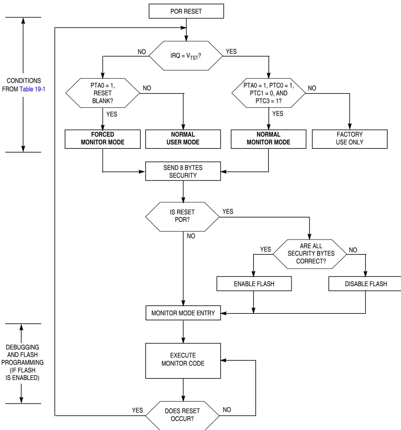
Figure 19-9. Simplified Monitor Mode Entry Flowchart
