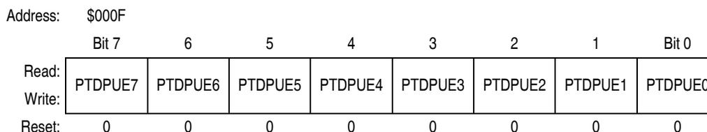
**Figure 12-16. Port D Input Pullup Enable Register (PTDPUE)**
