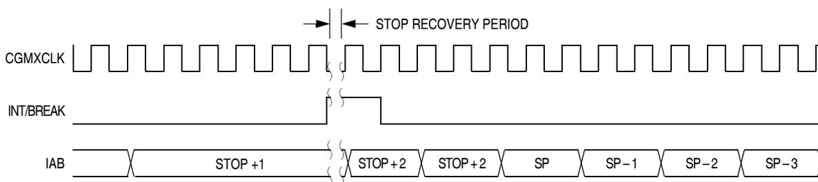
**Figure 15-19. Stop Mode Recovery from Interrupt**
