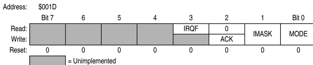
**Figure 8-4. IRQ Status and Control Register (INTSCR)**
