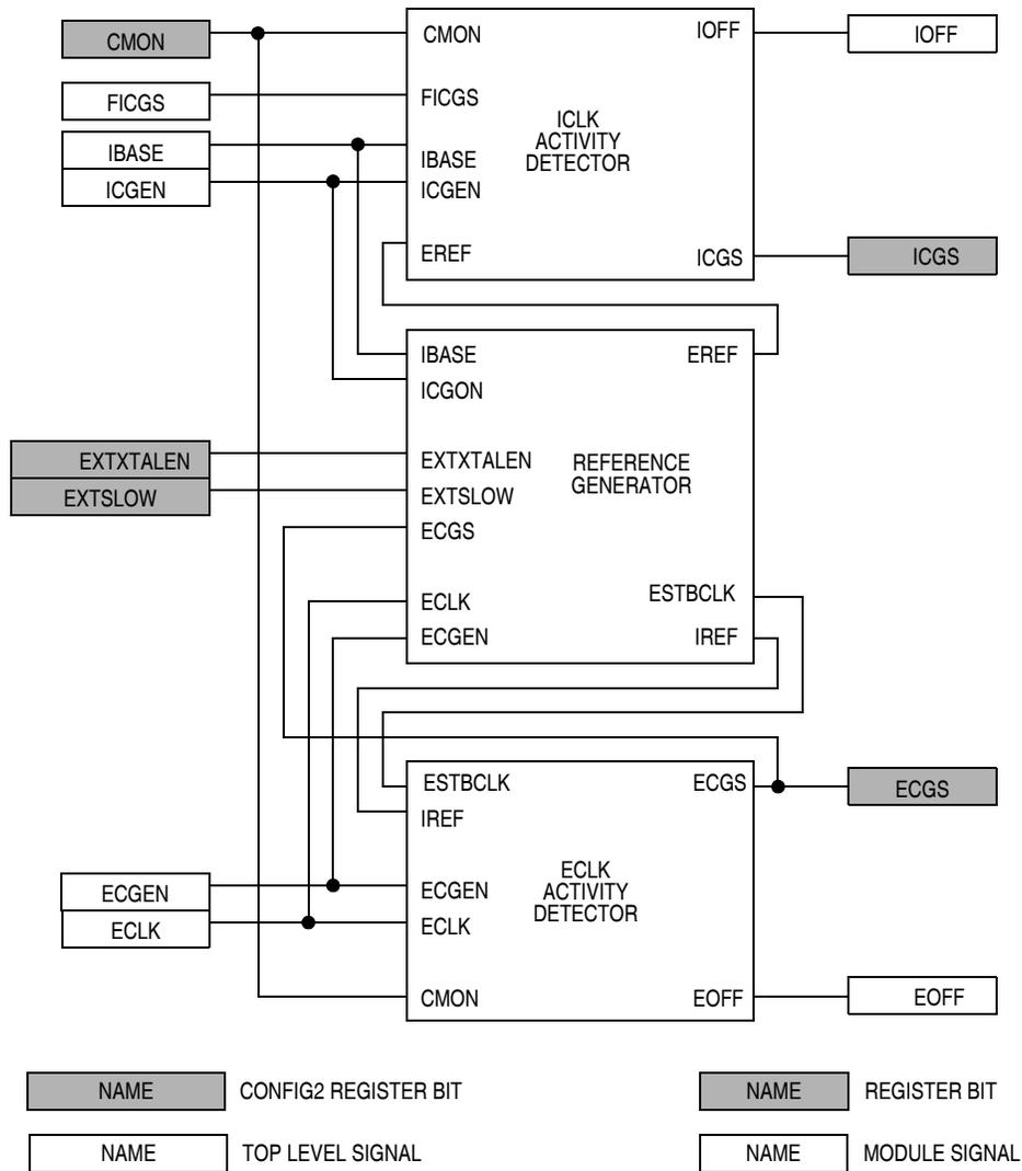
**Figure 7-5. Clock Monitor Block Diagram**
