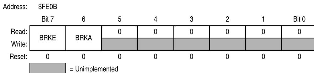
**Figure 19-4. Break Status and Control Register (BRKSCR)**
