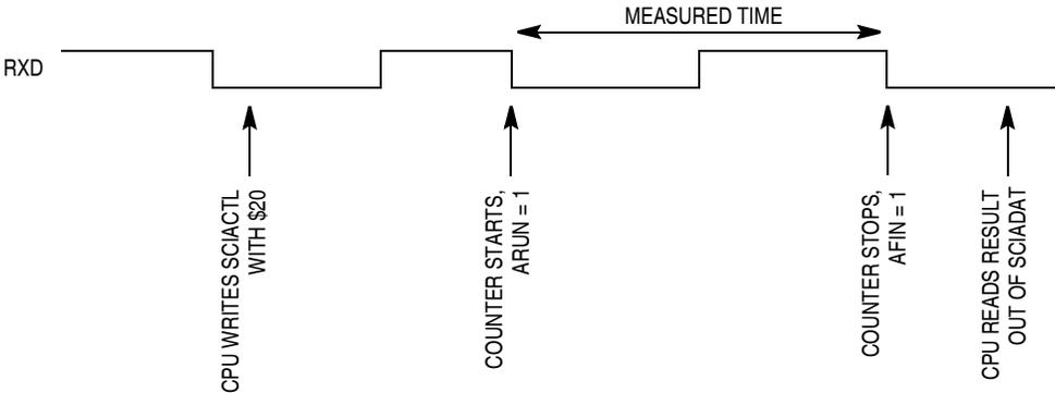
Figure 14-21. Bit Time Measurement with ACLK = 0
