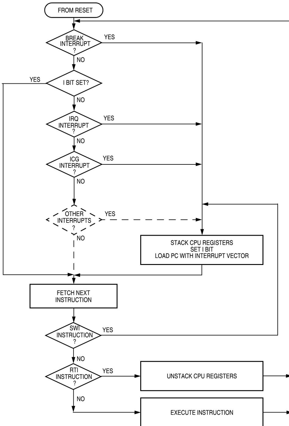
**Figure 13-6. Interrupt Processing**
