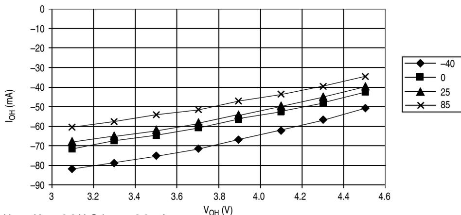
$V_{OH} > V_{DD} - 0.8 \text{ V} @ I_{OH} = -2.0 \text{ mA}$
