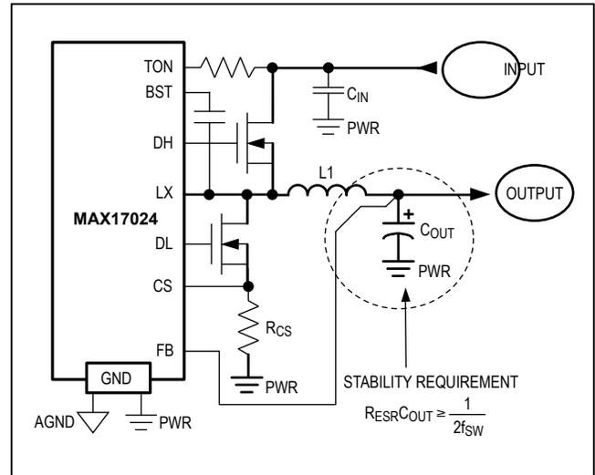
Figure 6. Standard Application with Output Polymer or Tantalum
