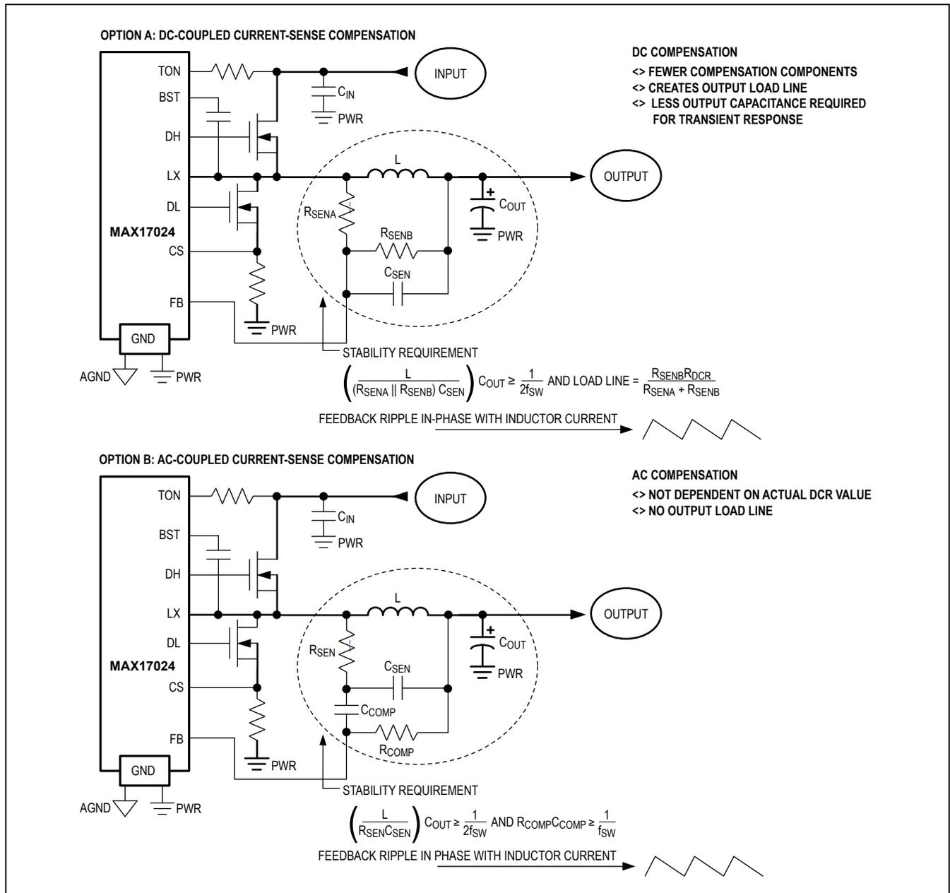
Figure 8. Feedback Compensation for Ceramic Output Capacitors
