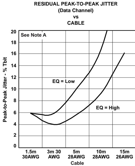
A. 1080p 10-Bit,  $V_{CC} = AV_{CC} = 3.3$  V,  $T_A = 25^\circ\text{C}$ ,  $R_{VSADJ} = 4.02$  k $\Omega$ , See Figure 5, Clock Channel = 185.6 MHz, Data Channel = 1.856 Gbps
