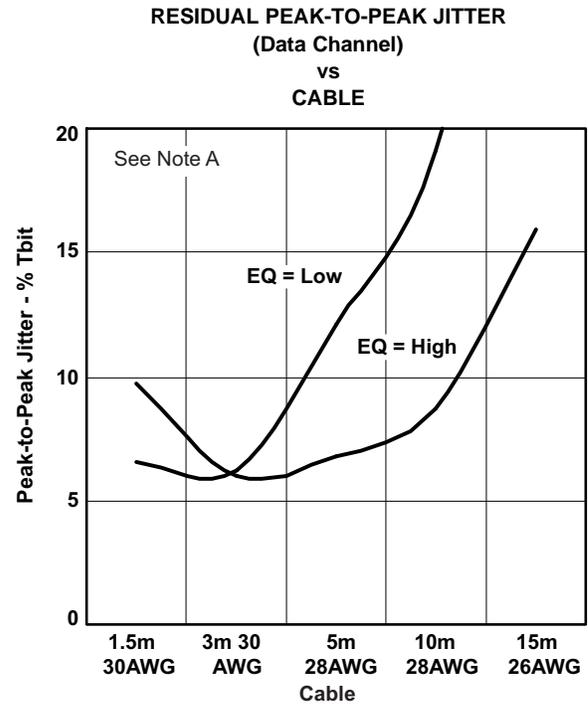
A. 1080p 12-Bit,  $V_{CC} = AV_{CC} = 3.3$  V,  $T_A = 25^\circ\text{C}$ ,  $R_{VSADJ} = 4.02$  k $\Omega$ , See Figure 5, Clock Channel = 222.8 MHz, Data Channel = 2.228 Gbps
