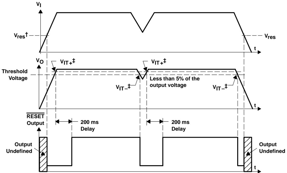
†  $V_{res}$  is the minimum input voltage for a valid  $\overline{\text{RESET}}$ . The symbol  $V_{res}$  is not currently listed within EIA or JEDEC standards for semiconductor symbology.
