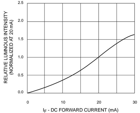
**Fig. 2 Relative Luminous Intensity vs. DC Forward Current**
