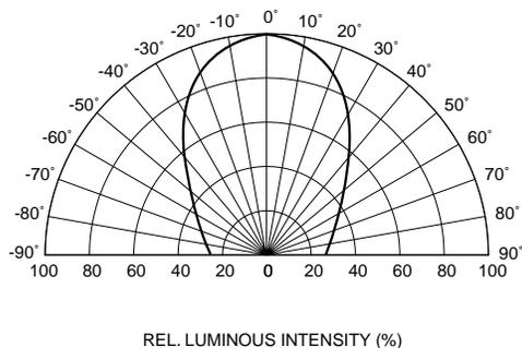
**Fig. 5A Radiation Diagram
