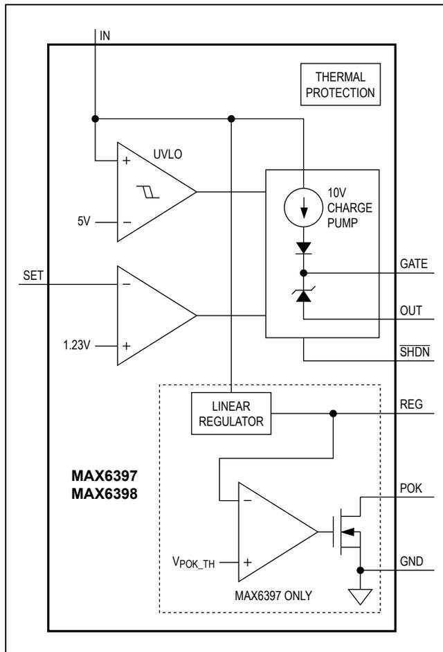
Figure 1. Functional Diagram
