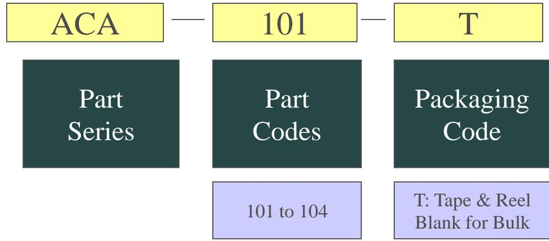
The ACA Series offers a range of Chip Antennas identified by part codes starting 101 to 104.
