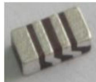
Chip Antennas are small ceramic blocks onto which silver patterns are printed to create an antenna structure. The term Chip Antenna covers a range of types of antenna offering different gains and layout considerations.
