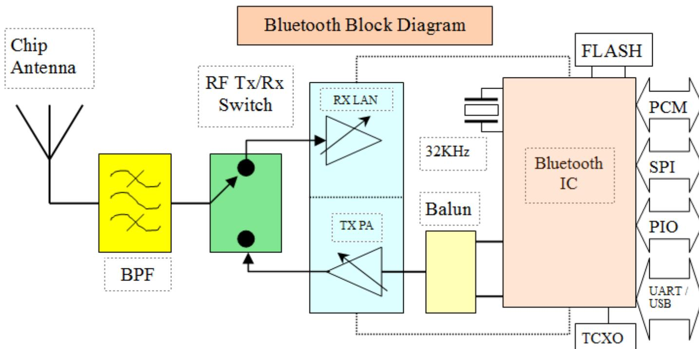
Block diagram shows application of **Chip Antenna** in the 2.45GHz Bluetooth TCVR. See also use of BPF, Balun, TCXO and 32.768KHz Xtal in Bluetooth module.
