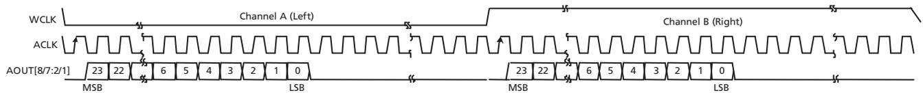
**Figure 4-26: I<sup>2</sup>S Audio Output Format**
