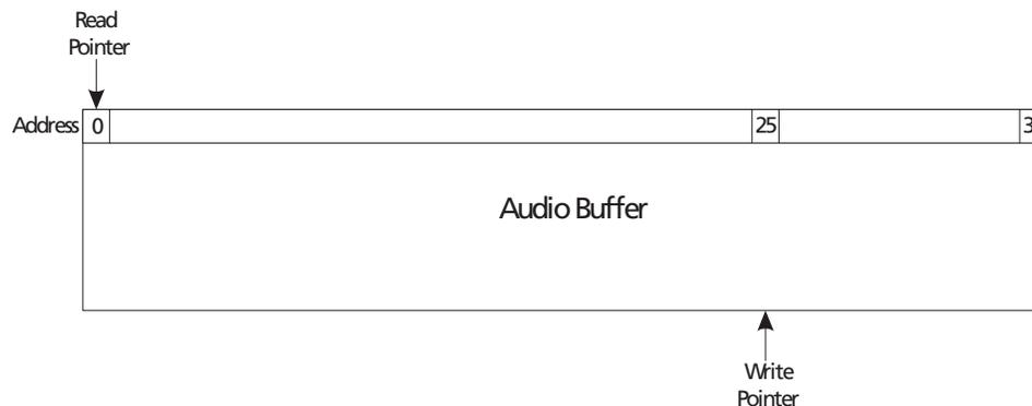
Figure 4-35: Audio Buffer After Initial 26 Sample Write
