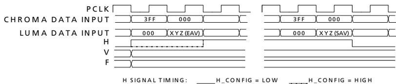
Figure 4-9: H:V:F Output Timing - SD 20-bit Output Mode
