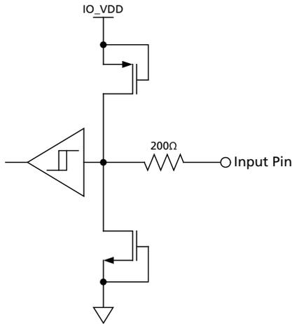
Figure 3-1: Digital Input Pin with Schmitt Trigger (20bit/ $\overline{10}$ bit,  $\overline{\text{AUDIO\_EN/DIS}}$ ,  $\overline{\text{CS\_TMS}}$ ,  $\overline{\text{SW\_EN}}$ ,  $\overline{\text{IOPROC\_EN/DIS}}$ ,  $\overline{\text{JTAG/HOST}}$ ,  $\overline{\text{RC\_BYP}}$ ,  $\overline{\text{RESET\_TRST}}$ ,  $\overline{\text{SCLK\_TCK}}$ ,  $\overline{\text{SDIN\_TDI}}$ ,  $\overline{\text{SDO\_EN/DIS}}$ ,  $\overline{\text{STANDBY}}$ ,  $\overline{\text{TIM\_861}}$ )
