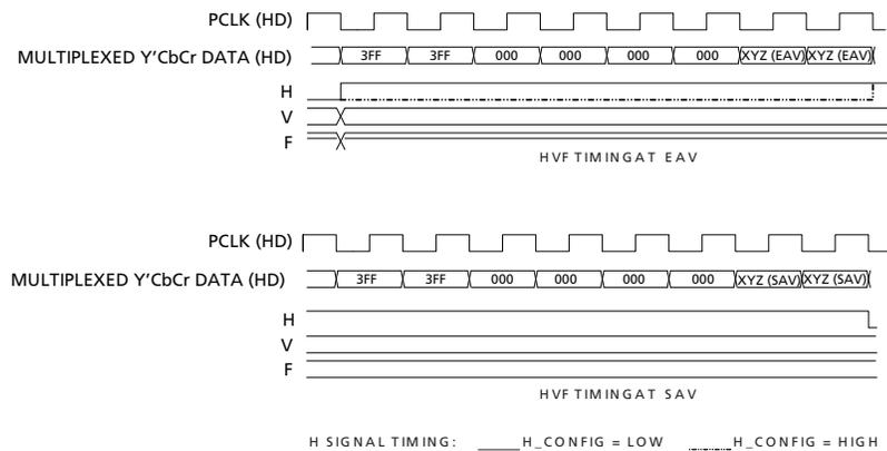
**Figure 4-6: H:V:F Output Timing - HDTV 10-bit Mode**
