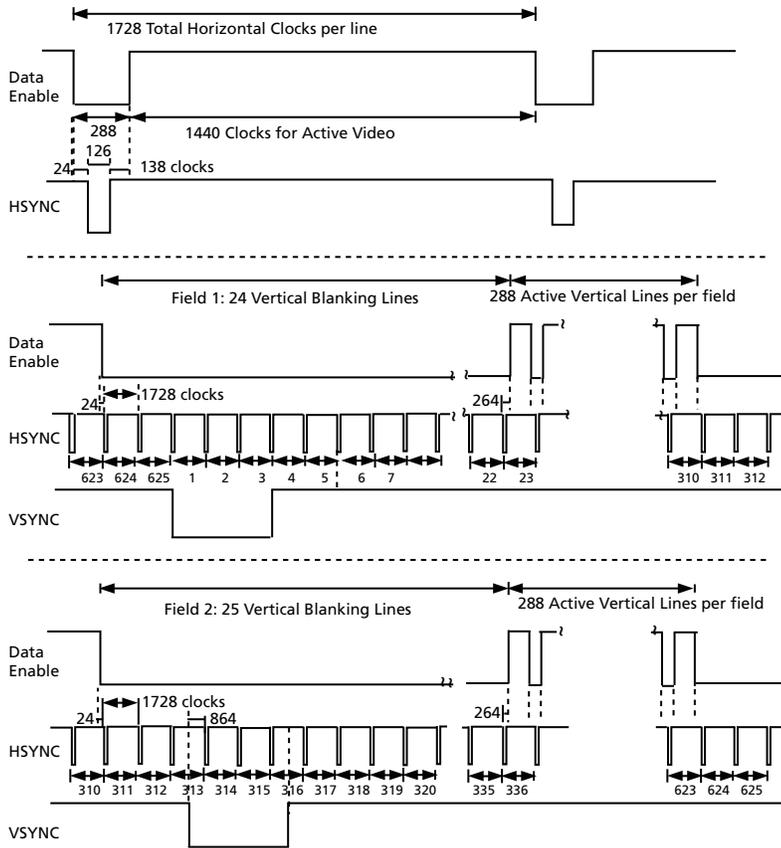
Figure 4-16: H:V:DE Output Timing 720 (1440) x 576 @ 50 (Format 21 & 22)
