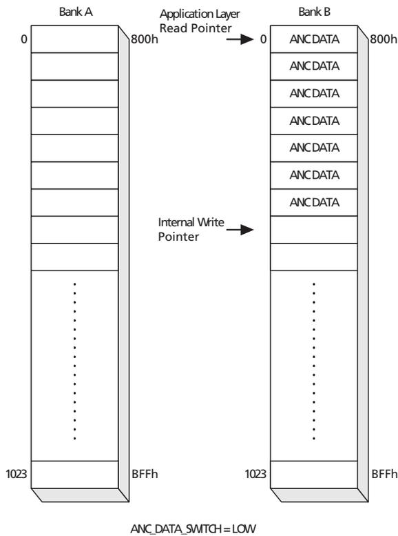
Figure 4-23: Ancillary Data Extraction - Step C
