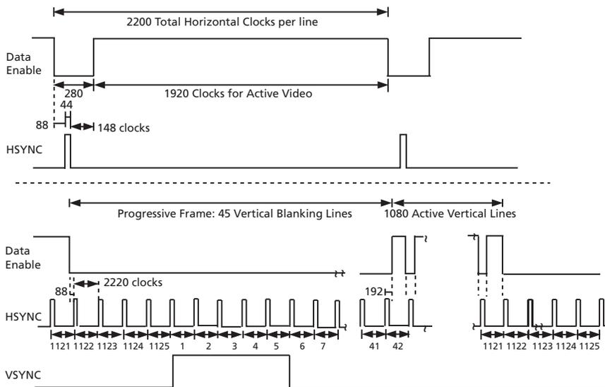
Figure 4-19: H:V:DE Output Timing 1920 x 1080p @ 29.97/30 (Format 34)
