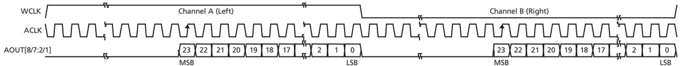
Figure 4-30: Serial Audio, Right Justified, MSB First
