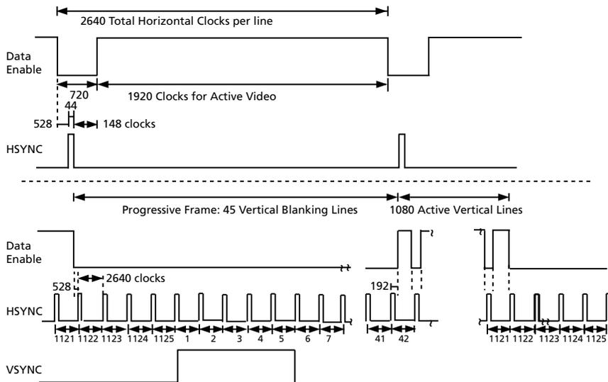
Figure 4-18: H:V:DE Output Timing 1920 x 1080p @ 25 (Format 33)
