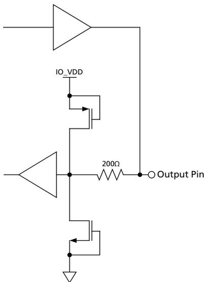
Figure 3-2: Bidirectional Digital Input/Output Pin - Configured to Output unless in Reset Mode. (ACLK, AMCLK, AOUT\_1/2, AOUT\_3/4, AOUT\_5/6, AOUT\_7/8, DVB\_ASI,  $\overline{\text{SMPTE\_BYPASS}}$ , WCLK)
