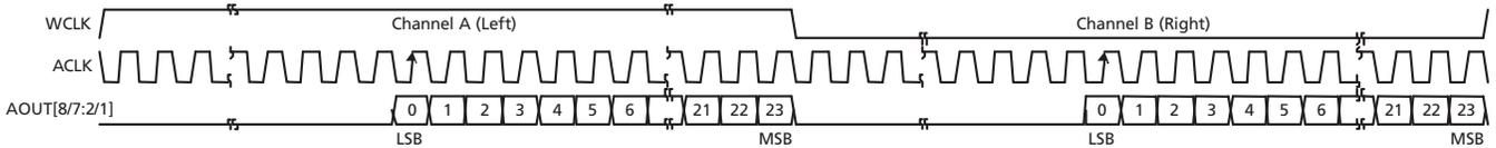
Figure 4-31: Serial Audio, Right Justified, LSB First
