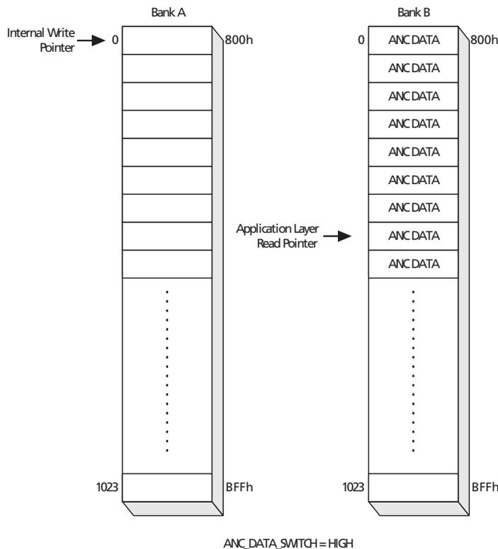
Figure 4-24: Ancillary Data Extraction - Step D
