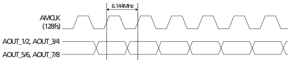
Figure 4-32: AES/EBU Audio Output to Bit Clock Timing
