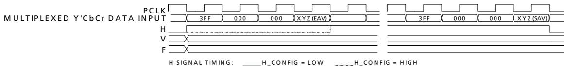
Figure 4-10: H:V:F Output Timing - SD 10-bit Output Mode
