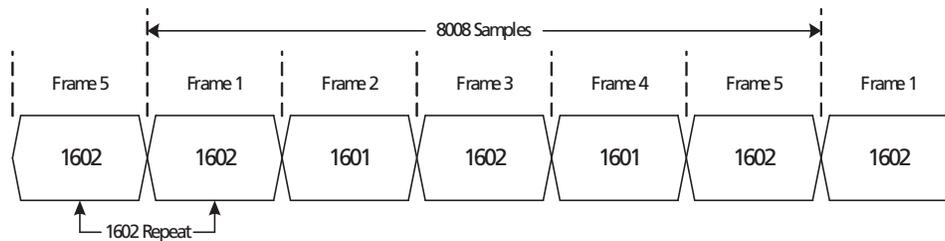
Figure 4-34: Sample Distribution over 5 Video Frames (525-line Systems)
