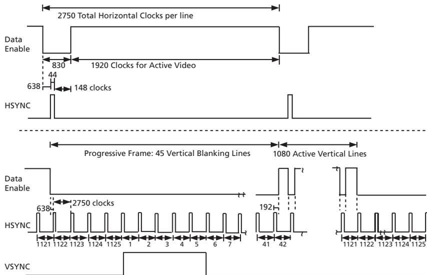
Figure 4-17: H:V:DE Output Timing 1920 x 1080p @ 23.94/24 (Format 32)
