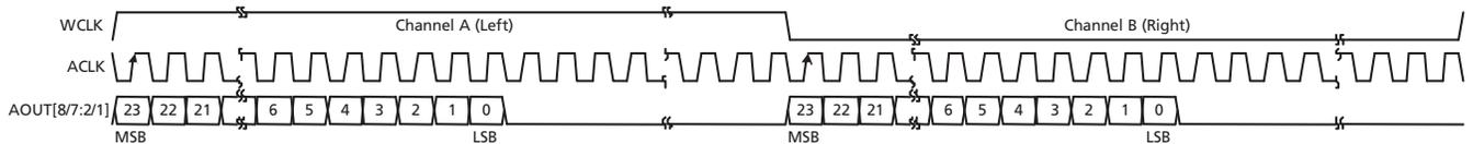
**Figure 4-28: Serial Audio, Left Justified, MSB First**
