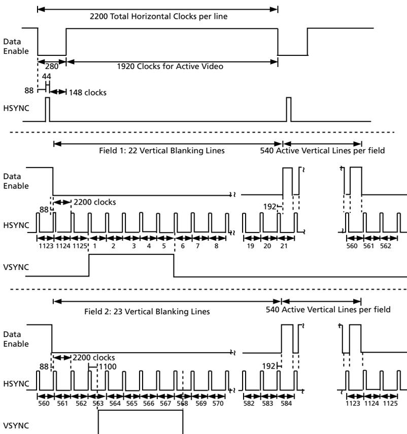
Figure 4-12: H:V:DE Output Timing 1920 x 1080i @ 59.94/60 (Format 5)
