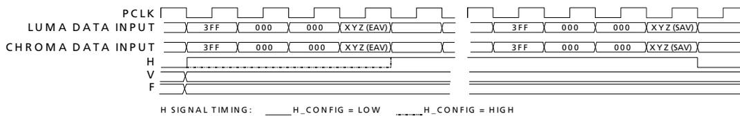
Figure 4-7: H:V:F Output Timing - HD 20-bit Output Mode
