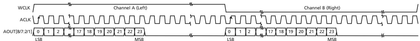
**Figure 4-29: Serial Audio, Left Justified, LSB First**
