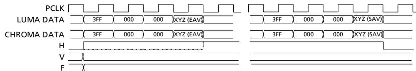
**Figure 4-5: H:V:F Output Timing - HDTV 20-bit Mode**
