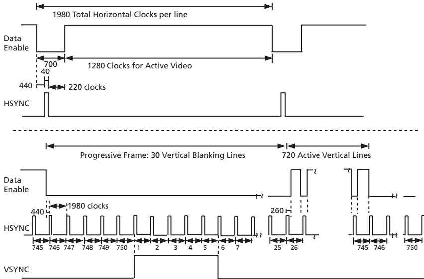
Figure 4-14: H:V:DE Output Timing 1280 x 720p @ 50 (Format 19)
