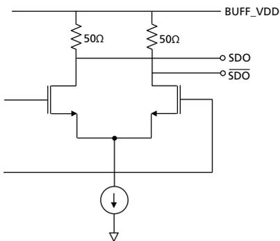
Figure 3-9: SDO/ $\overline{\text{SDO}}$
