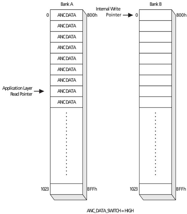
Figure 4-22: Ancillary Data Extraction - Step B
