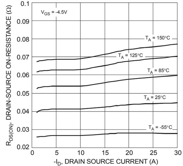
Figure 12 Typical On-Resistance vs. Drain Current and Temperature
