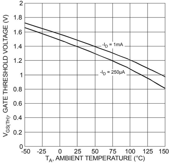
Figure 15 Gate Threshold Variation vs. Ambient Temperature
