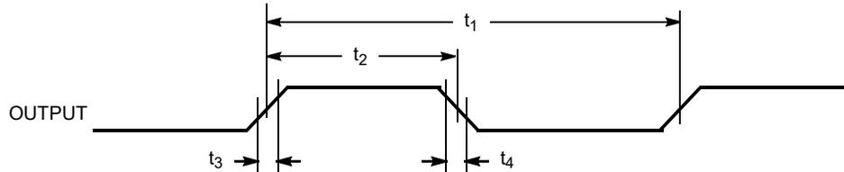
Figure 9. Output Tristate Timing
