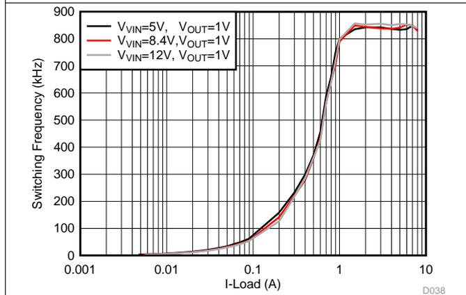
Figure 23.  $F_{SW}$  Load Regulation, Eco-mode,  $F_{SW} = 800\text{ kHz}$
