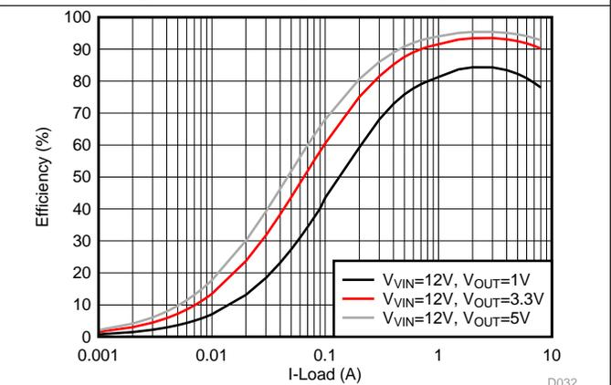
**Figure 18. Efficiency, FCCM,  $F_{SW} = 1\text{ MHz}$**
