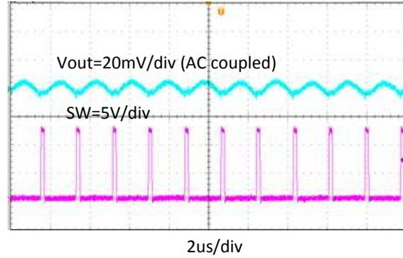
Figure 38. Output Voltage Ripple,  $I_{OUT} = 8\text{ A}$
