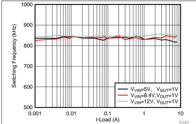
Figure 25.  $F_{SW}$  Load Regulation, FCCM,  $F_{SW} = 800$  kHz
