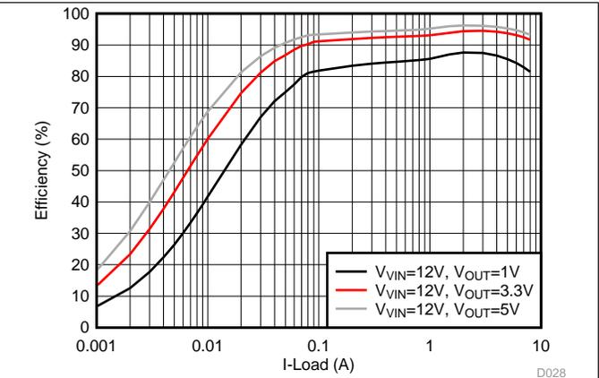
**Figure 14. Efficiency, OOA-mode,  $F_{SW} = 600\text{ kHz}$**
