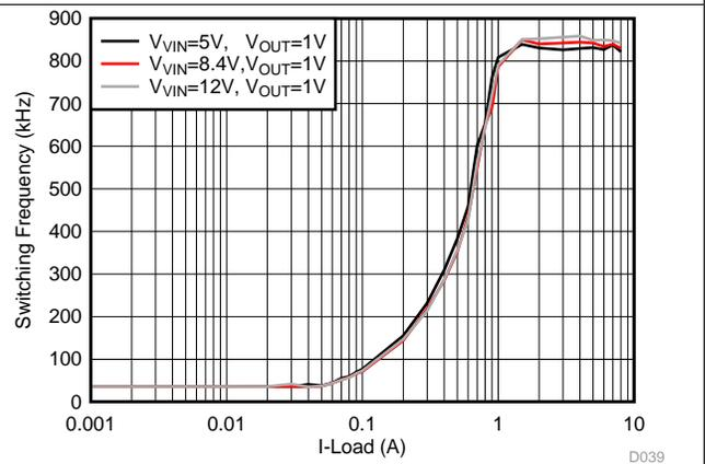
Figure 24.  $F_{SW}$  Load Regulation, OOA-mode,  $F_{SW} = 800\text{ kHz}$
