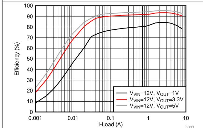
**Figure 17. Efficiency, OOA-mode,  $F_{SW} = 1\text{ MHz}$**
