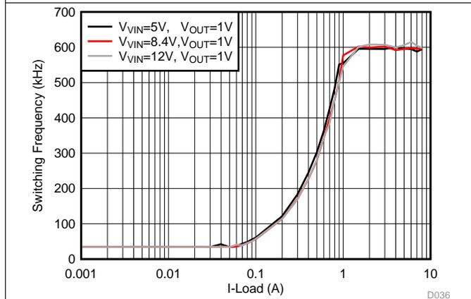
Figure 21.  $F_{SW}$  Load Regulation, OOA-mode,  $F_{SW} = 600\text{ kHz}$
