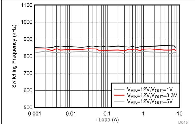
Figure 27.  $F_{SW}$  Load Regulation, FCCM,  $F_{SW} = 800$  kHz
