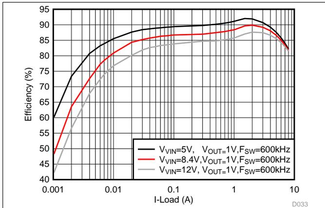
Figure 31. Efficiency Curve
