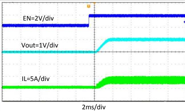
Figure 39. Start-Up Through EN,  $I_{OUT} = 4\text{ A}$
