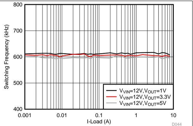
Figure 26.  $F_{SW}$  Load Regulation, FCCM,  $F_{SW} = 600$  kHz
