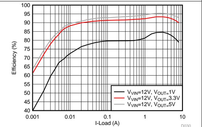
**Figure 16. Efficiency, Eco-mode,  $F_{SW} = 1\text{ MHz}$**
