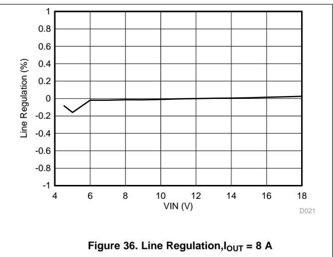
Figure 36. Line Regulation,  $I_{OUT} = 8\text{ A}$
