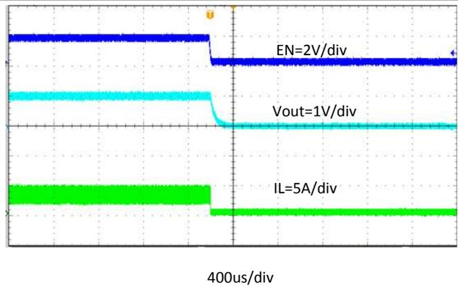
Figure 40. Shut-down Through EN,  $I_{OUT} = 4\text{ A}$
