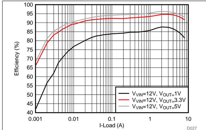
**Figure 13. Efficiency, Eco-mode,  $F_{SW} = 600\text{ kHz}$**
