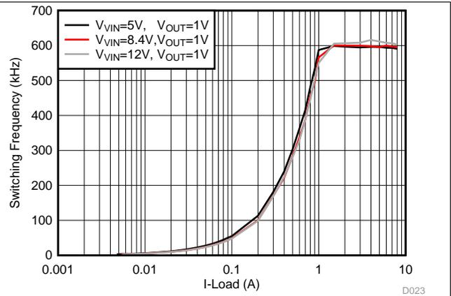
Figure 20.  $F_{SW}$  Load Regulation, Eco-mode,  $F_{SW} = 600\text{ kHz}$
