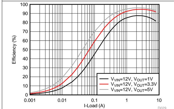
**Figure 15. Efficiency, FCCM,  $F_{SW} = 600\text{ kHz}$**
