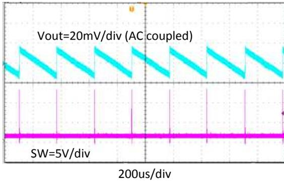
Figure 37. Output Voltage Ripple,  $I_{OUT} = 0.01\text{ A}$
