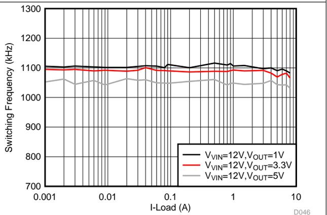
Figure 28.  $F_{SW}$  Load Regulation, FCCM,  $F_{SW} = 1$  MHz
