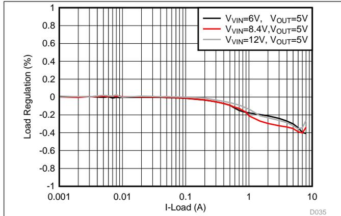
Figure 19. Load Regulation, Eco-mode,  $F_{SW} = 600\text{ kHz}$
