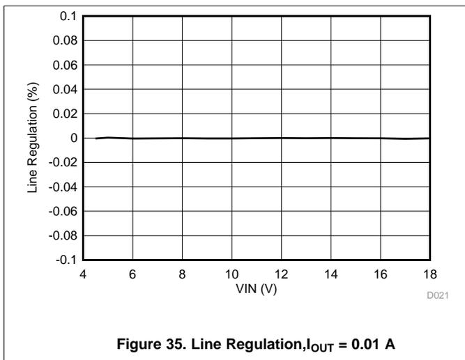
Figure 35. Line Regulation,  $I_{OUT} = 0.01\text{ A}$
