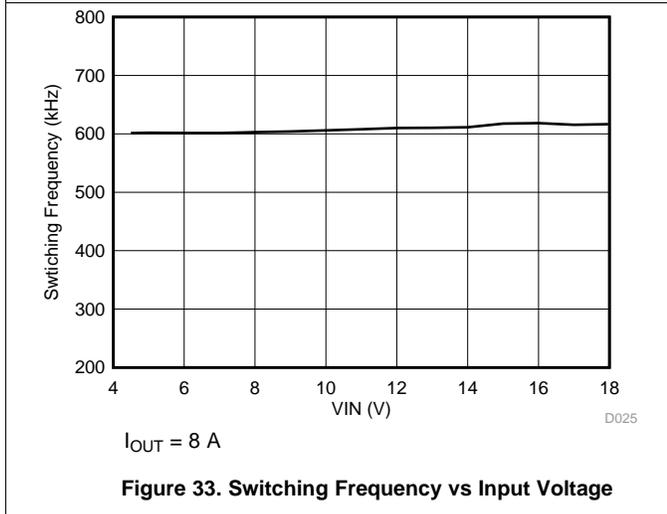
Figure 33. Switching Frequency vs Input Voltage
