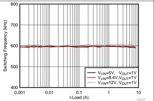
Figure 22.  $F_{SW}$  Load Regulation, FCCM,  $F_{SW} = 600\text{ kHz}$
