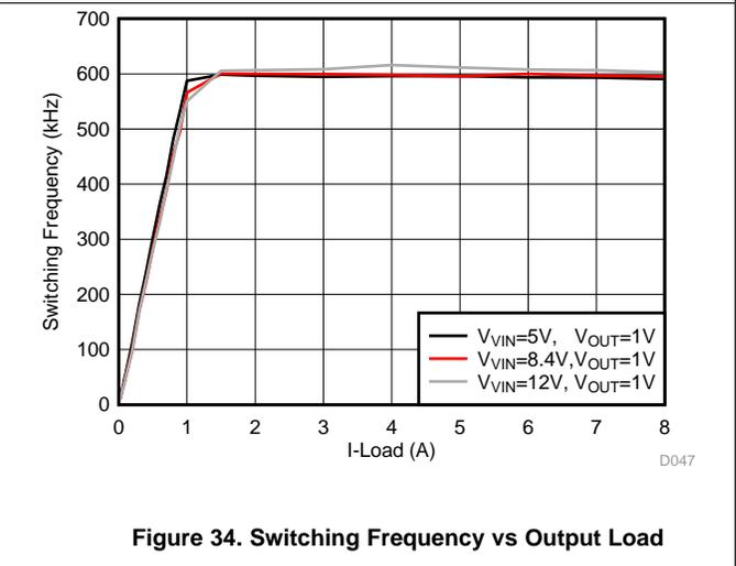
Figure 34. Switching Frequency vs Output Load
