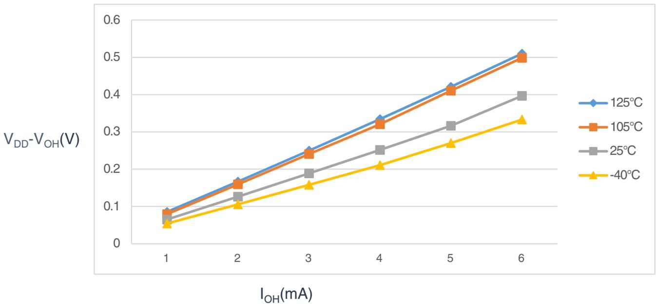
**Figure 2. Typical I<sub>OH</sub> Vs. V<sub>DD</sub>-V<sub>OH</sub> (standard drive strength) (V<sub>DD</sub> = 5 V)**
