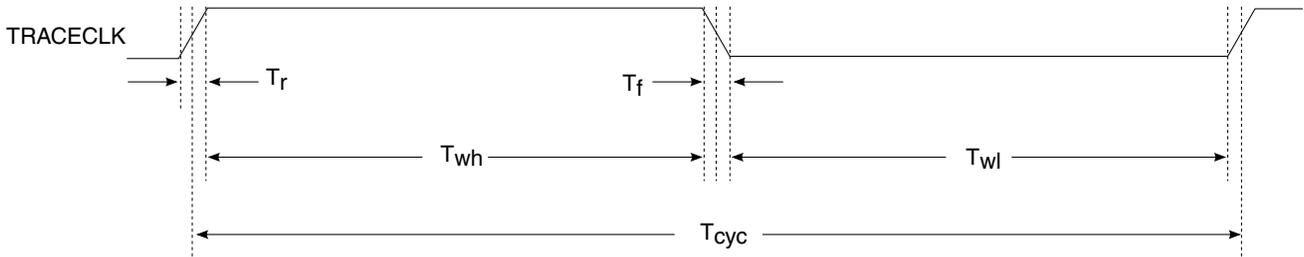
Figure 12. TRACE\_CLKOUT specifications
