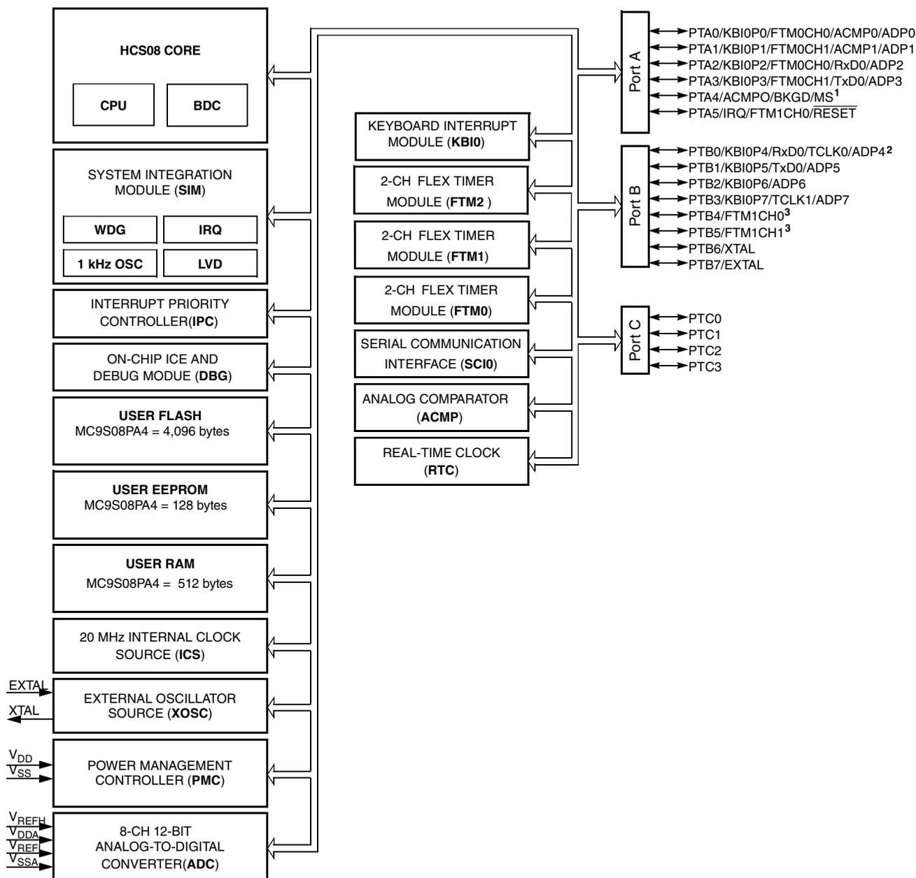
1. PTA4/ACMP0/BKGD/MS is an output-only pin when used as port pin.
