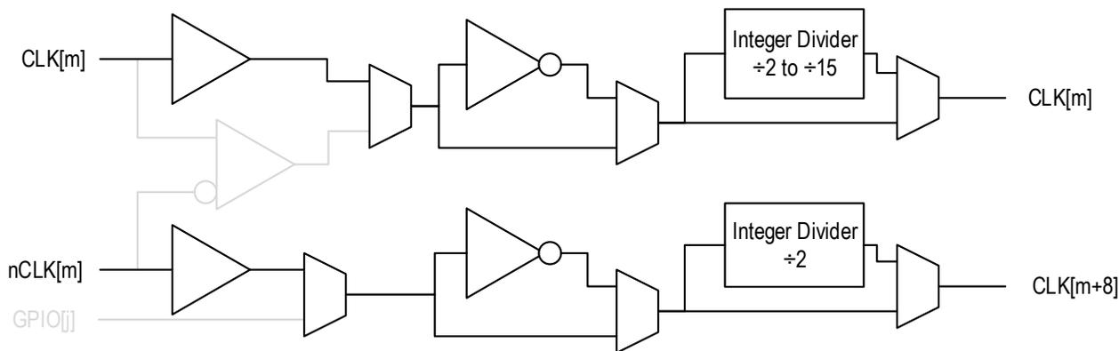
When programmed as differential plus one single-ended as shown in [Figure 7](#), two independent inputs are provided to the 8A34041. This mode can only be used with the GPIOs and input stages shown in [Table 5](#).
