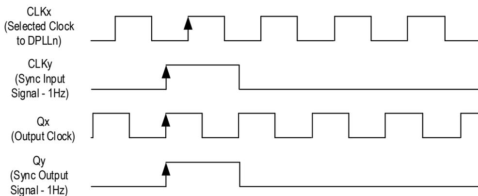
In [Figure 9](#), CLKx is the associated input clock and CLKy is the sync pulse, and they are both input to DPLLn. Qx is the output clock that is locked to CLKx, and Qy is the output sync pulse output of DPLLn.
