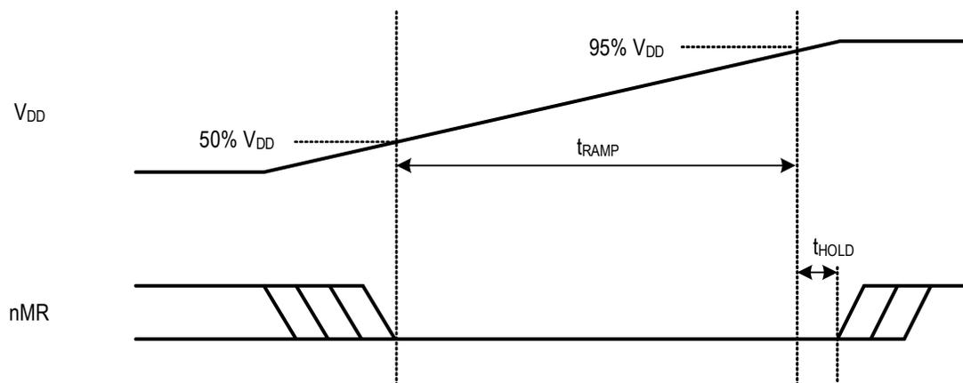
In cases where the device is not powering up and just being reset, a low pulse on nMR of 20ns will be sufficient to reset the device.
