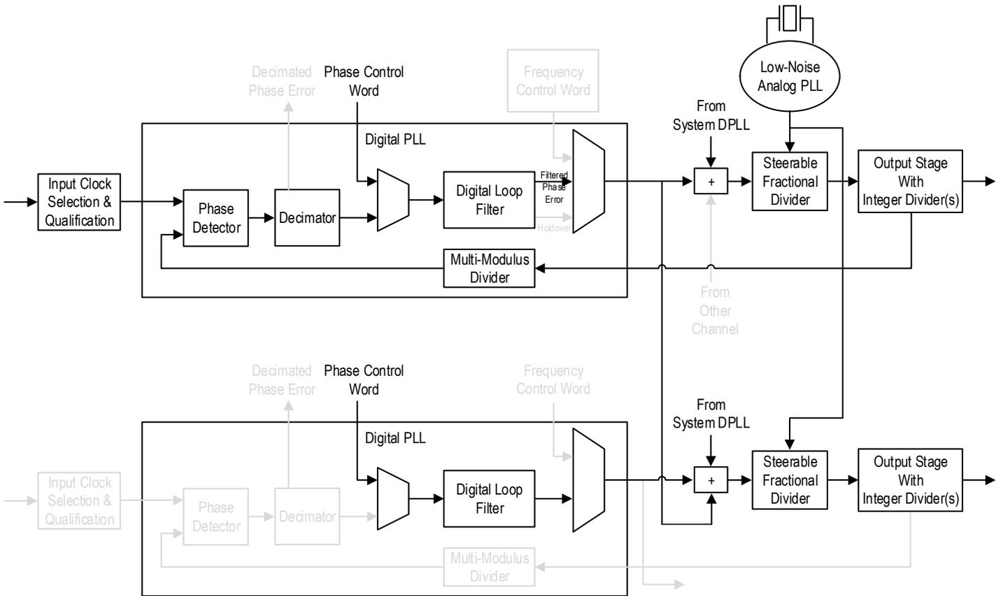
In this example, the IEEE 1588 timestamps are used to calculate the phase offset between the IEEE 1588 master's 1PPS pulse and the IEEE 1588 slave's 1PPS pulse and then align the two pulses by moving the slave's 1PPS pulse in phase. The slave must be able to move the 1PPS pulse by  $\pm 0.5s$ , and the 8A34041 provides this capability.
