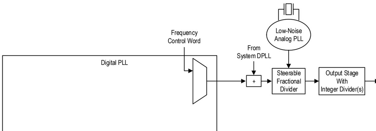
The FCW is a 42-bit 2's-complement value. The FCW has a granularity of  $1.11 \times 10^{-10}$  ppm and a full range of +244.20ppm to -244.08ppm of the nominal DCO frequency. A positive value will increase the output frequency and a negative one will decrease the output frequency. The formula for calculation of the FCW from the fractional frequency offset (FFO) is:
