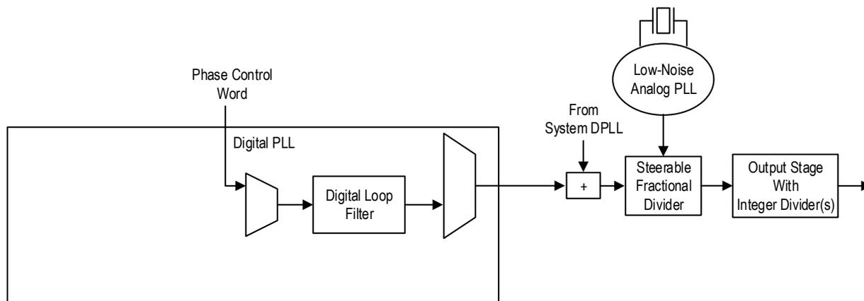
To assist in the above, there is an optional timer associated with the PCW. This allows a phase control word to be applied for a limited period of time after which it will be automatically reset to zero or placed into holdover by the 8A34041, and therefore, it will avoid the DCO continuing to apply the phase adjustment indefinitely until it reaches its tuning range limits. The timer value is a 16-bit integer that has a granularity of 1 millisecond and a full range of up to 65.535 seconds.
