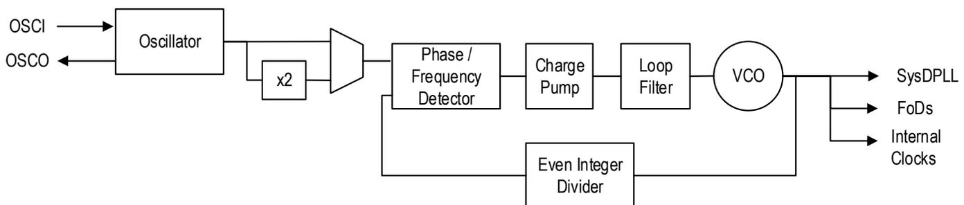
During a device reset, the APLL is configured by loading the appropriate control register fields from the internal One-Time Programmable memory or an external serial EEPROM, whichever is enabled and has valid contents. After the reset sequence has completed, the APLL can be re-configured manually over the serial port at any time.
