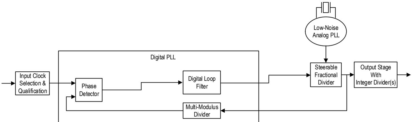
The high-frequency output signal from the APLL is divided-down by the FOD block to a frequency from 500MHz to 1GHz. The output frequency is unrelated to the APLL frequency since fractional division is used (for information, see System Analog PLL (APLL)). That signal is in turn fed to the output stage, where it is further divided by the integer divider(s) and provided to the output in the selected output format. For more information, see FOD Multiplexing and Output Stages.
