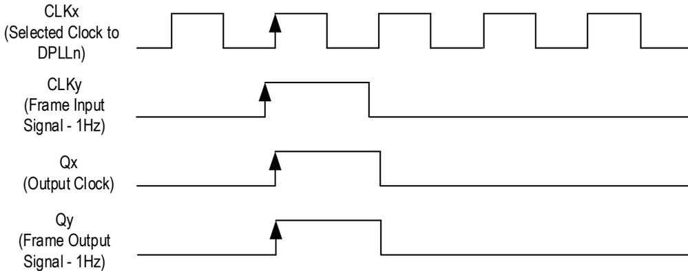
In [Figure 8](#), CLKx is the associated input clock and CLKy is the frame pulse, and they are both input to DPLLn. Qx is the output clock that is locked to CLKx, and Qy is the output frame pulse output of DPLLn.
