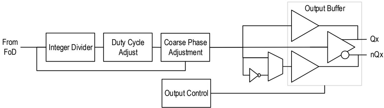
Other than having two copies of each functional block fed from the same FOD, both single and dual output stages behave the same. Similarly, the two paths within the dual output stages behave the same as each other. Descriptions of each functional block are provided in the following sub-sections.
