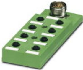
Sensor/actuator box, Connection method: M12 socket Plastic, Number of slots: 6, Number of positions: 5, Slot assignment: Double, Status indication: No, Universal; Master cable connection: M23 plug connection 90°, Shielding: No
