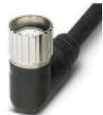
Female connector, Number of positions: 19, Status indication: No; Master cable connection: M23 socket, Cable length: 10 m, Shielding: No
