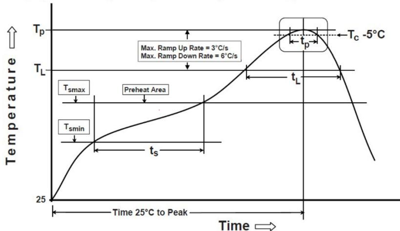
**Note :** All temperature measurement points are on top/surface of the component. If temperature exceeds the recommended, it will cause surface peeling or damage.
