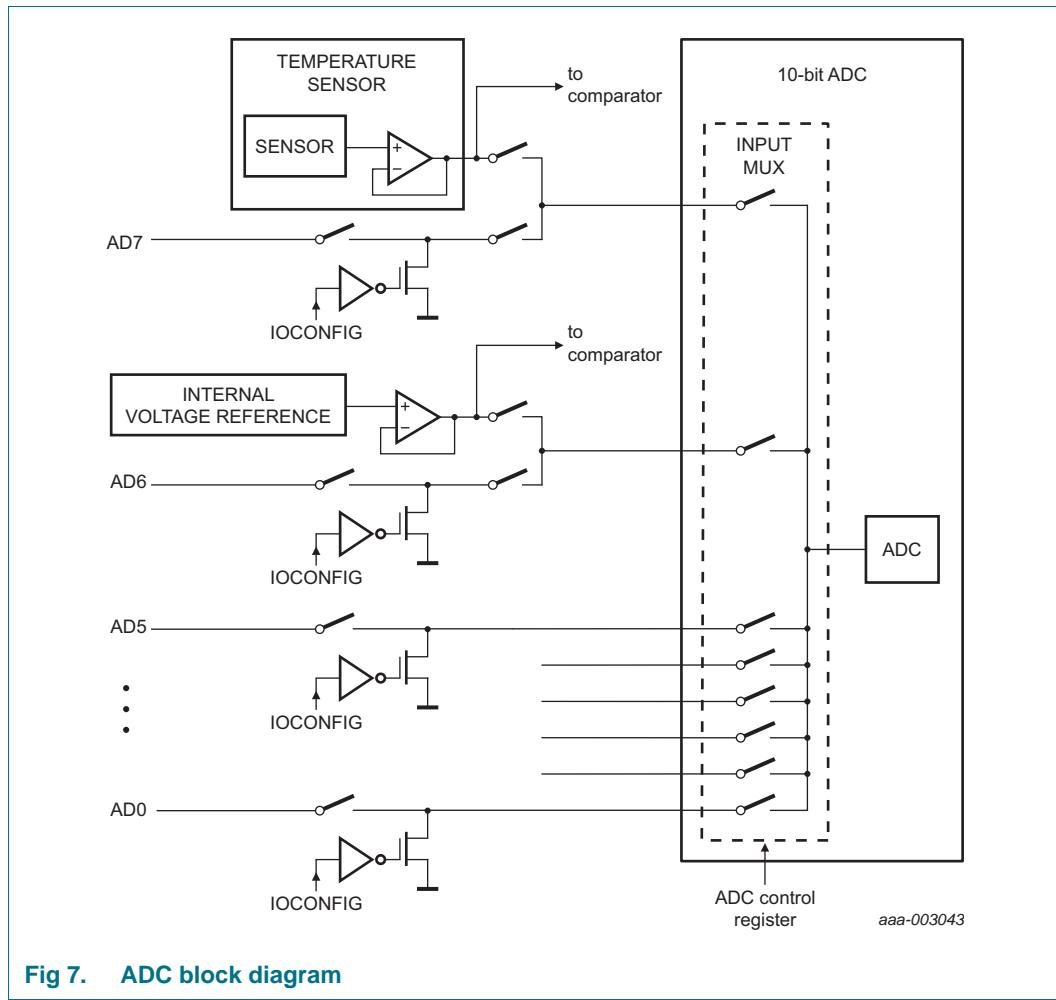
Fig 7. ADC block diagram
