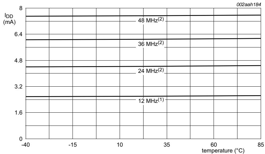
Conditions:  $V_{DD(3V3)} = 3.3$  V; active mode entered executing code while(1){ } from flash; all peripherals disabled in the SYSAHBCLKCTRL register; all peripheral clocks disabled; all analog peripherals disabled in the PDRUNCFG register; low-current mode (see [Section 7.22.6.2](#)).
