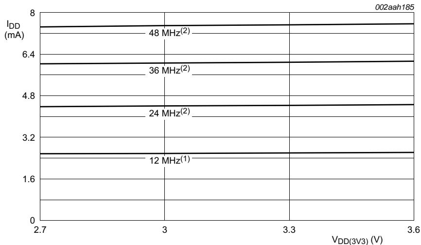
Conditions:  $T_{amb} = 25^{\circ}\text{C}$ ; active mode entered executing code while(1){ } from flash; all peripherals disabled in the SYSAHBCLKCTRL register; all peripheral clocks disabled; all analog peripherals disabled in the PDRUNCFG register; low-current mode (see [Section 7.22.6.2](#)).
