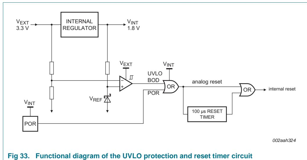
Fig 33. Functional diagram of the UVLO protection and reset timer circuit
