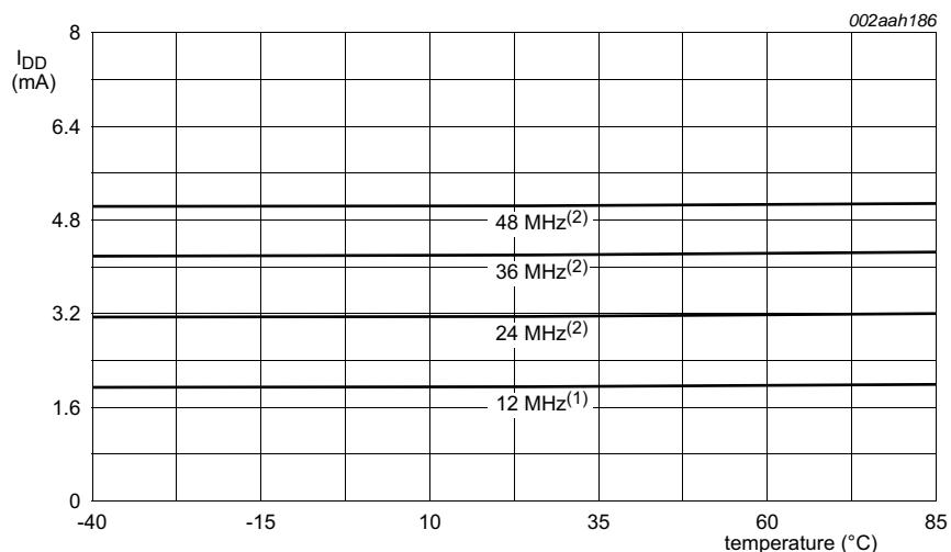
Conditions:  $V_{DD(3V3)} = 3.3\text{ V}$ ; sleep mode entered from flash; all peripherals disabled in the SYSAHBCLKCTRL register and PDRUNCFG register; all peripheral clocks disabled; BOD disabled; low-current mode (see [Section 7.22.6.2](#)).
