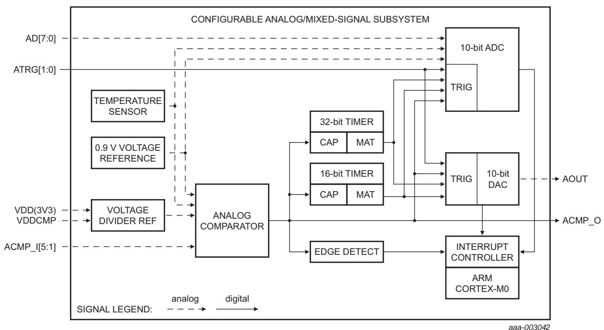
**Fig 6. Configurable analog/mixed signal subsystem**
