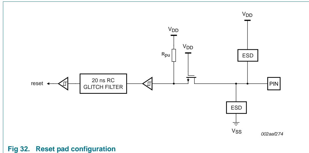
Fig 32. Reset pad configuration
