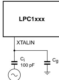
**Fig 29. Slave mode operation of the on-chip oscillator**
