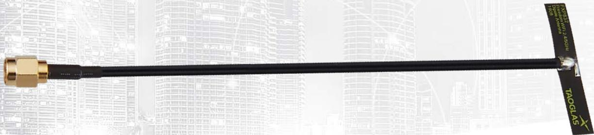
The Freedom FXP832 is a breakthrough, very high efficiency, small, dual-band Wi-Fi dipole omni-directional antenna for 2.4/5GHz bands. This antenna is designed for DSRC, V2V, Wi-Fi, Bluetooth, Zigbee and other applications in these bands. It is designed in such a narrow rectangular form factor to cover most of the current applications on the market. Taoglas FXP series are conformal flexible antennas and can fit irregular housings.
