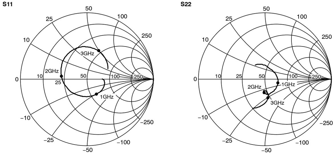
Figure 10. S Parameter ( $V_{CC} = 5\text{ V}$ )
