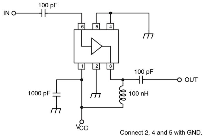
Figure 1. Test Circuit
