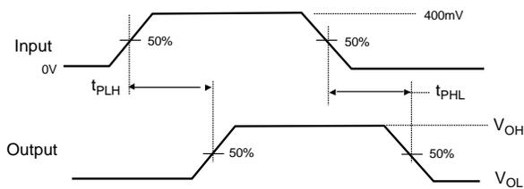
**Figure 7. Propagation Delay ( $t_{RTF} = 500$  ps)**
