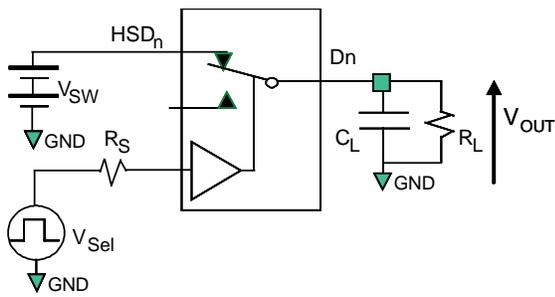
$R_L$ ,  $R_S$ , and  $C_L$  are functions of the application environment (see AC Tables for specific values)
