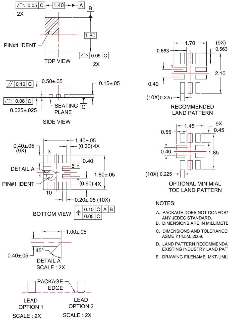
Figure 15. 10-Lead, Ultrathin Molded Leadless Package (UMLP)
