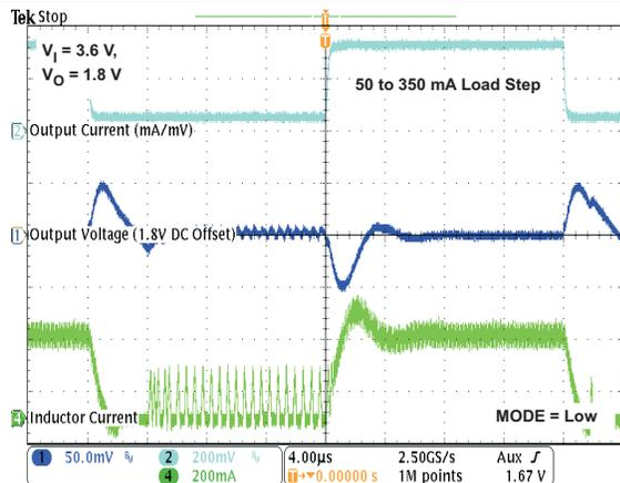
Figure 39. Load Transient Response in PFM/PWM Operation
