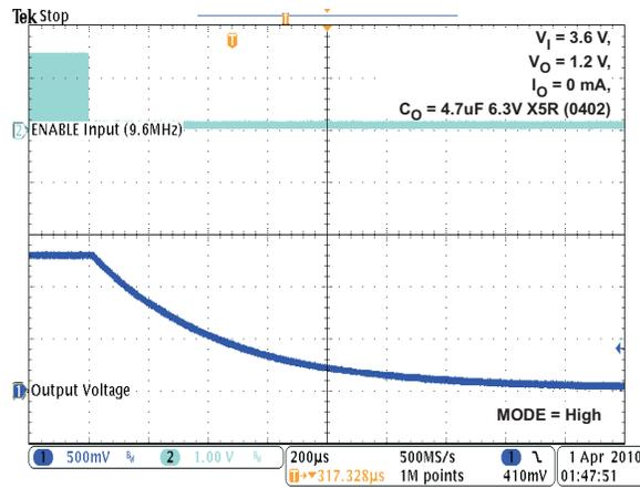
Figure 49. Shut-Down (RF Clock)
