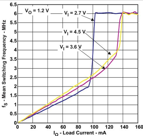
Figure 17. PFM Switching Frequency vs Input Voltage
