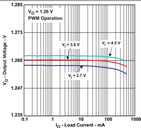
Figure 11. DC Output Voltage vs Load Current
