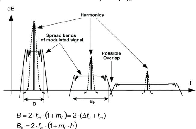
**Figure 27. Spread Bands of Harmonics in Modulated Square Signals <sup>(1)</sup>**
