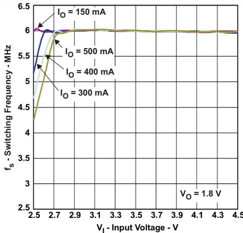
Figure 15. PWM Switching Frequency vs Input Voltage
