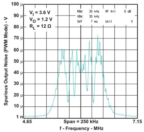
**Figure 20. Spurious Output Noise (PWM Mode) vs Frequency**
