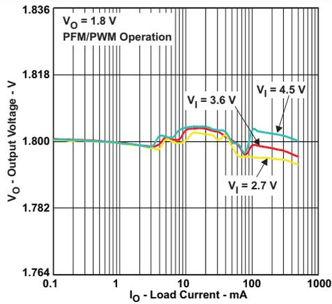
Figure 9. DC Output Voltage vs Load Current
