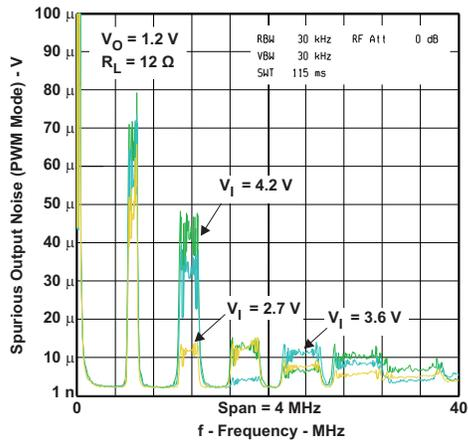
**Figure 19. Spurious Output Noise (PWM Mode) vs Frequency**
