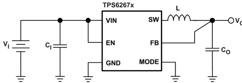
**Figure 24. Measurement Setup**
