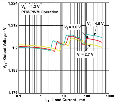
Figure 10. DC Output Voltage vs Load Current
