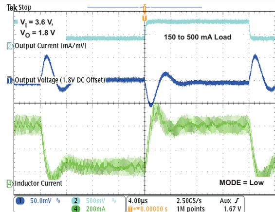
Figure 40. Load Transient Response in PWM/PWM Operation
