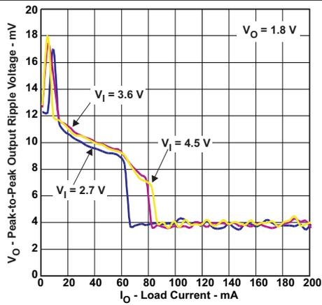
Figure 7. Peak-To-Peak Output Ripple Voltage vs Load Current
