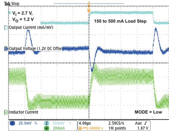
Figure 36. Load Transient Response in PWM/PWM Operation
