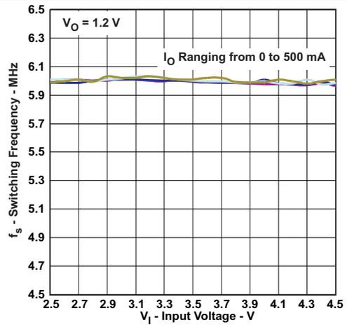
Figure 16. PWM Switching Frequency vs Input Voltage
