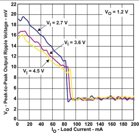
Figure 8. Peak-To-Peak Output Ripple Voltage vs Load Current
