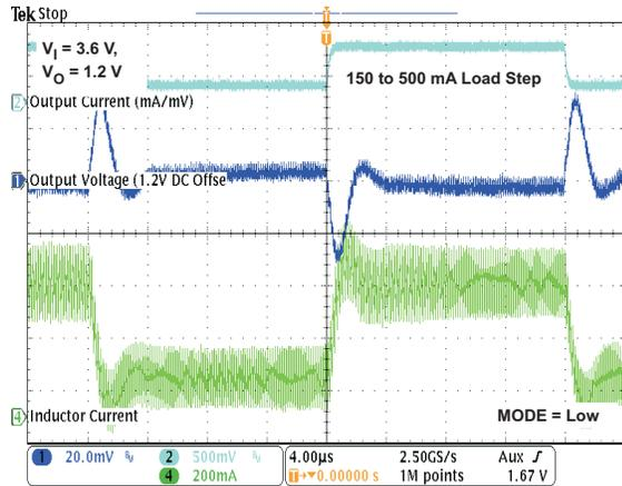
Figure 35. Load Transient Response in PWM/PWM Operation
