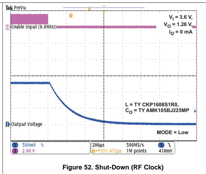
Figure 52. Shut-Down (RF Clock)
