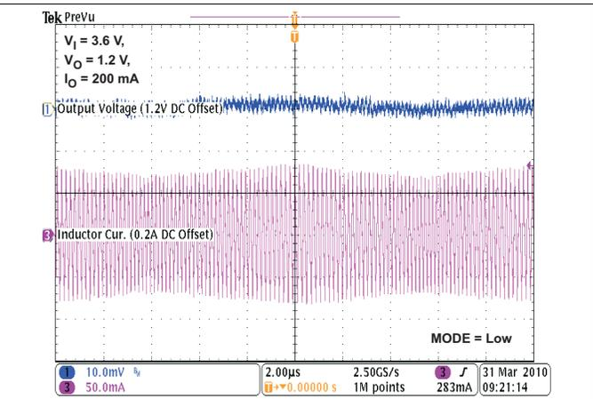
Figure 44. PWM Mode Operation - SSFM Modulation
