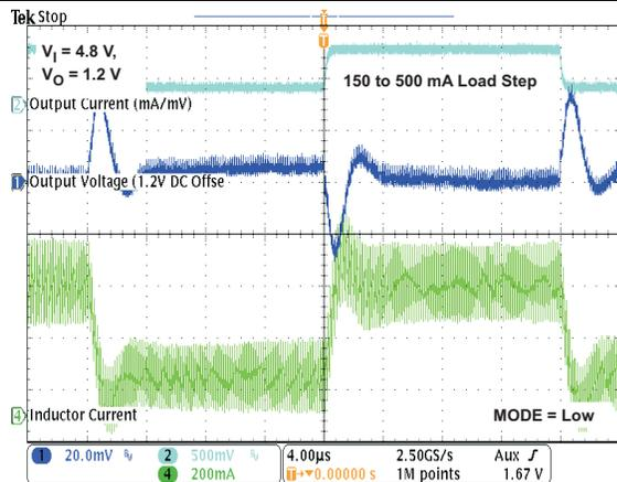
Figure 37. Load Transient Response in PWM/PWM Operation
