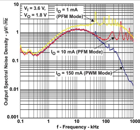
**Figure 23. Output Spectral Noise Density vs Frequency**
