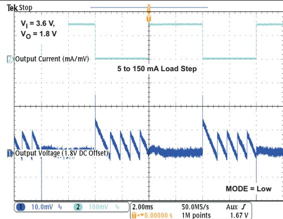
Figure 38. Load Transient Response in PFM/PWM Operation
