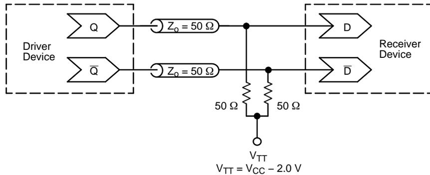
**Figure 2. Typical Termination for Output Driver and Device Evaluation**
