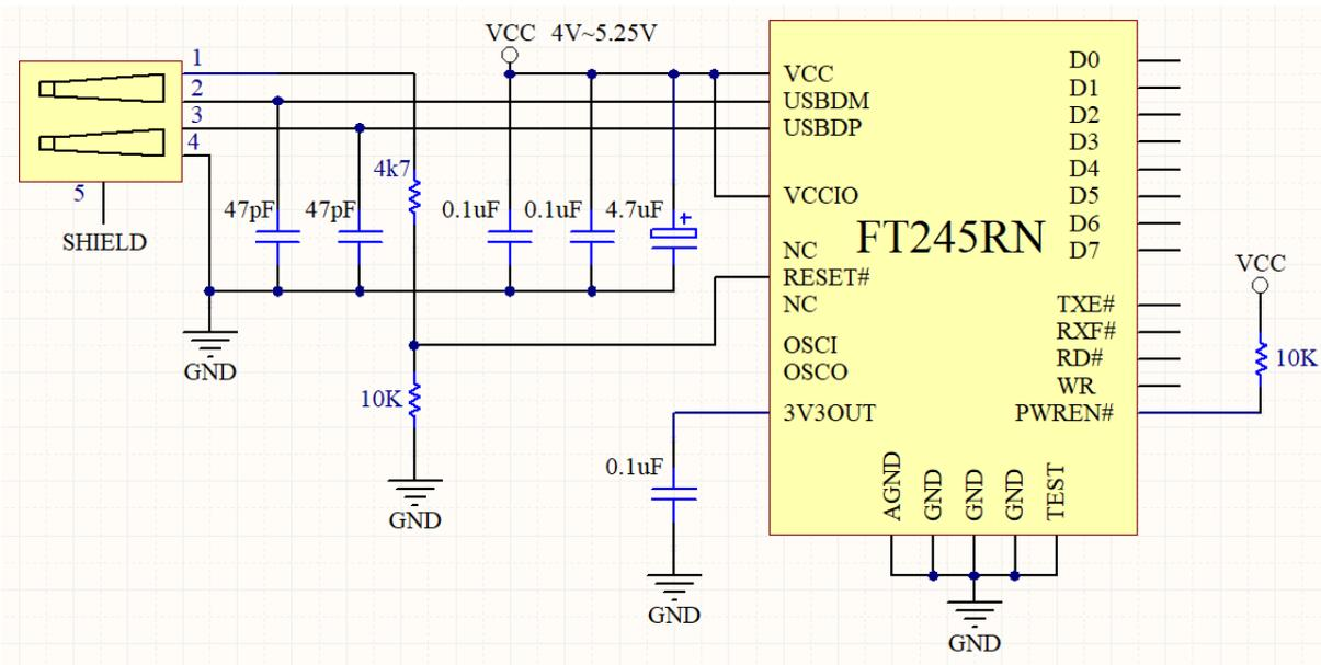
**Figure 6.2 Self-Powered Configuration**
