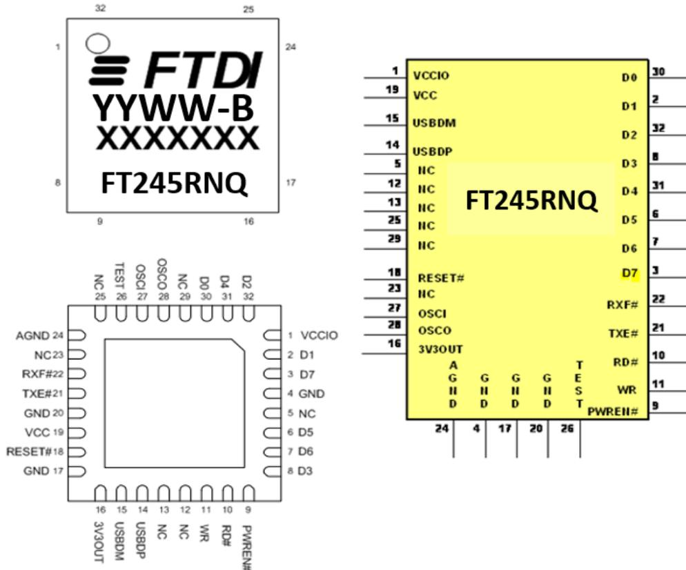
**Figure 3.2 QFN-32 Package Pin Out and schematic symbol**
