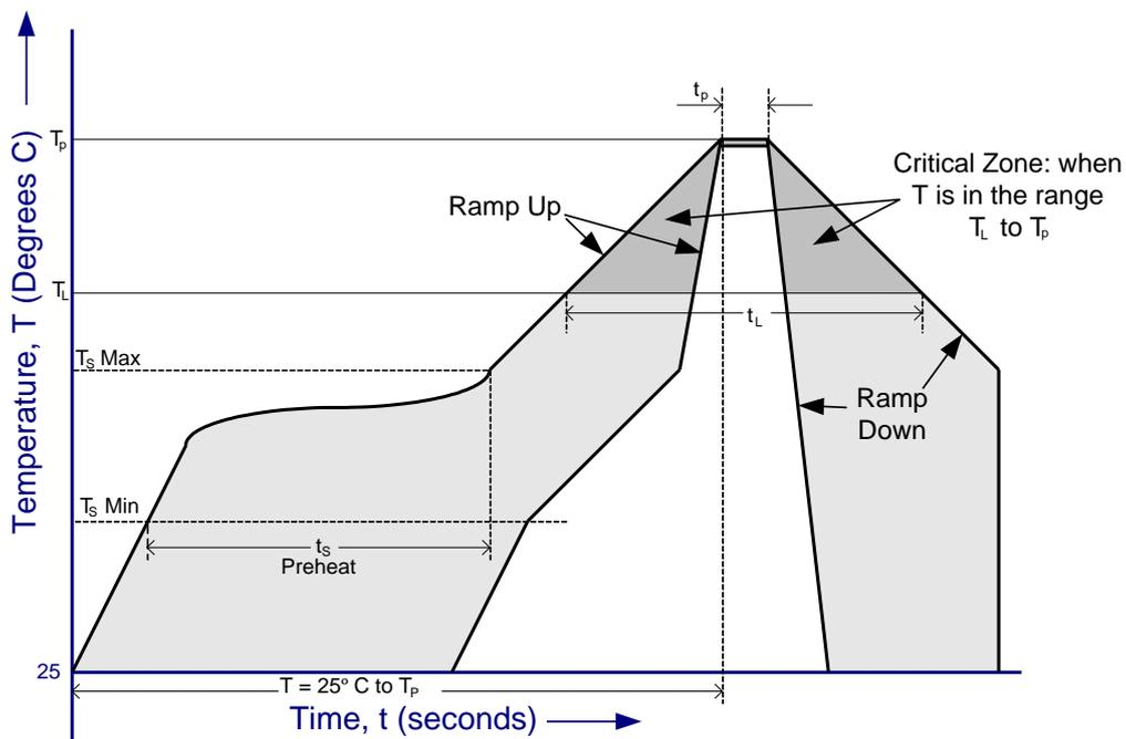
**Figure 9.3 FT245RN Solder Reflow Profile**
