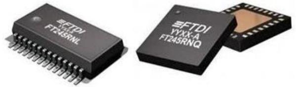
The FT245RN is a USB to parallel FIFO interface with the following advanced features:
