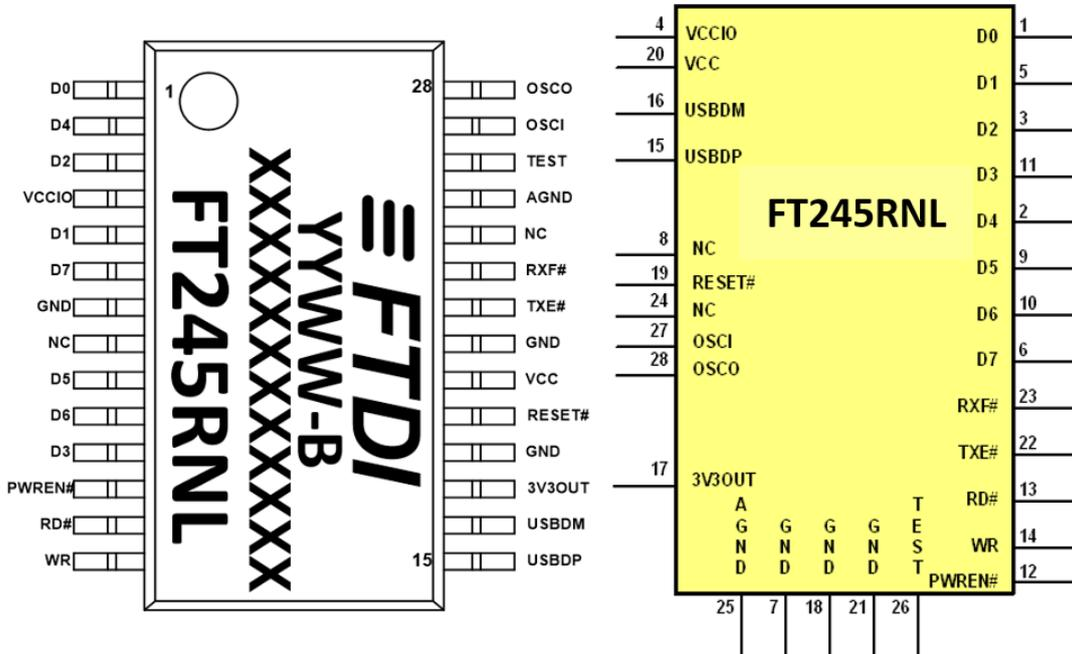
Figure 3.1 SSOP Package Pin Out and Schematic Symbol
