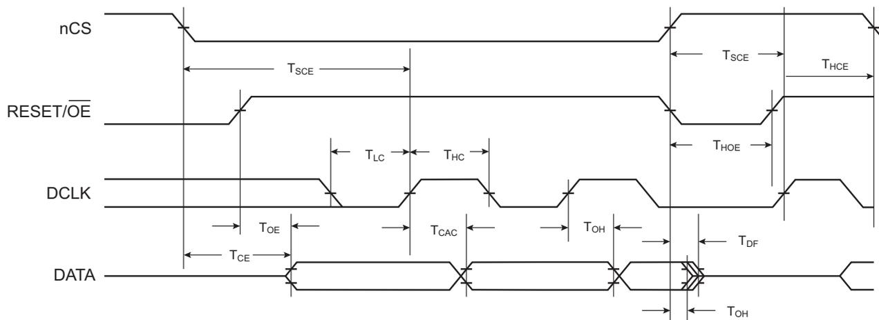
**Figure 10-2. AC Waveforms when Cascading**
