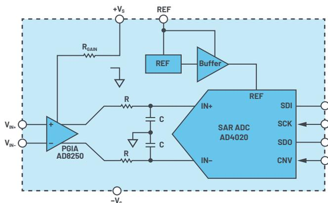
Figure 1. A simplified block diagram of a precise data acquisition system.
