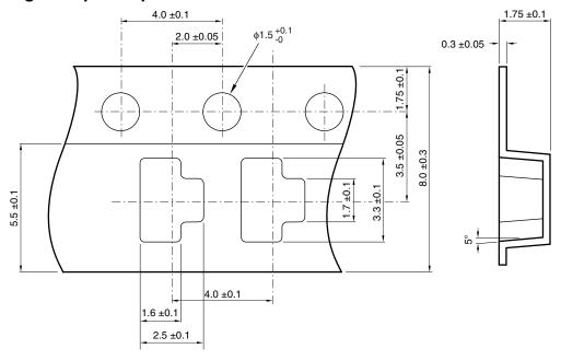
Fig. 6 Reel Shape and Dimension
