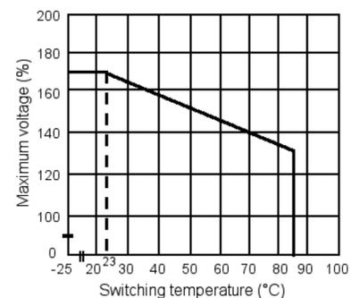
**Note:** The maximum coil voltage refers to the maximum value in a varying range of operating power voltage, not a continuous voltage.
