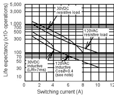
**Note:** Curve 120VAC inductive Cosφ=0.4 is same for 250VAC resistive load.
