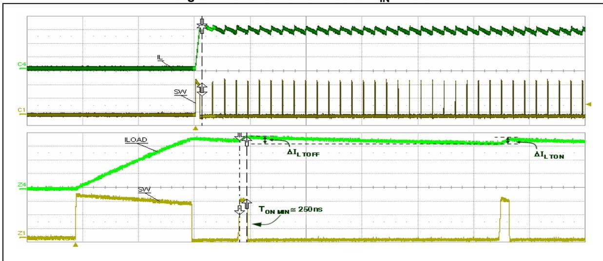
Figure 14. Short-circuit current  $V_{IN} = 24\text{ V}$
