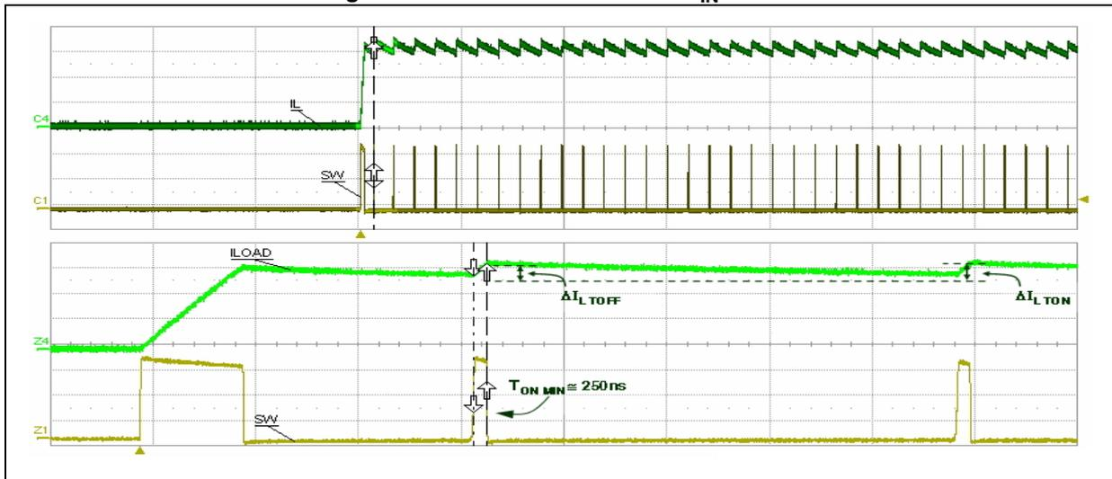
Figure 15. Short-circuit current  $V_{IN} = 36\text{ V}$
