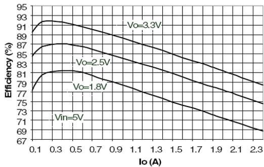
Figure 32. Efficiency vs output current -  $V_{IN} = 12\text{ V}$
