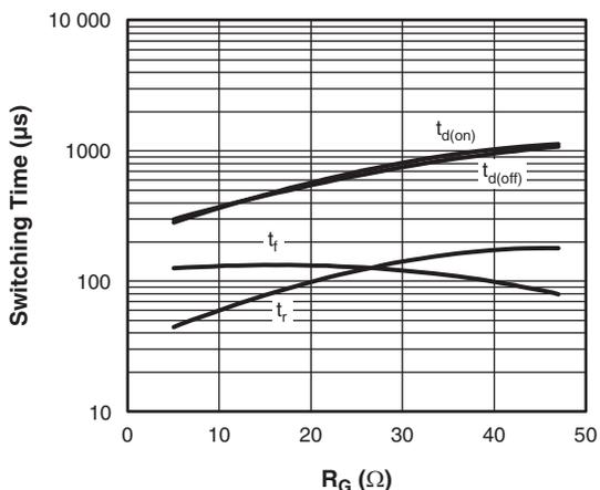
Fig. 12 - Typical IGBT Switching Time vs.  $R_g$
