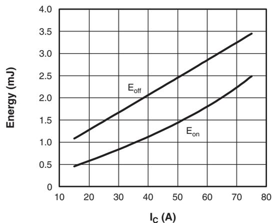
Fig. 9 - Typical IGBT Energy Loss vs.  $I_C$
