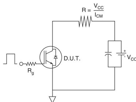
Fig. 17b - Pulsed Collector Current Test Circuit
