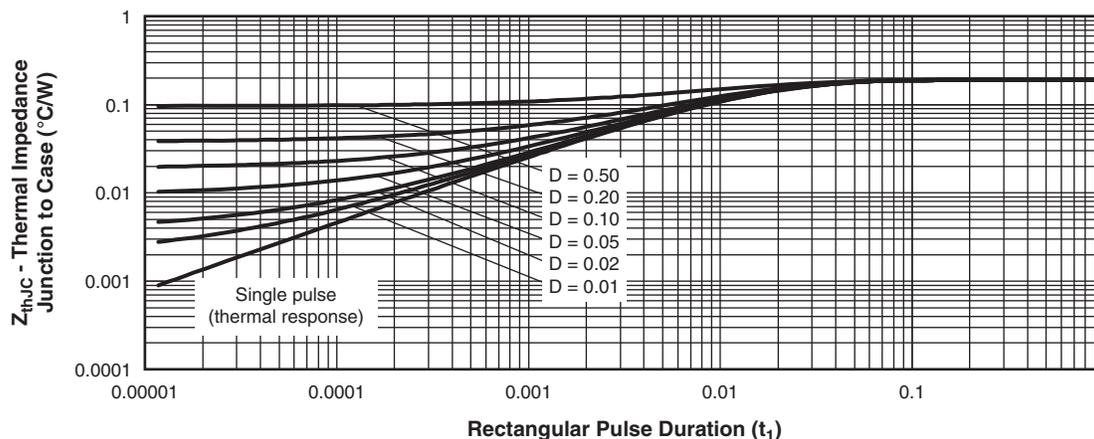
Fig. 15 - Maximum Thermal Impedance  $Z_{thJC}$  Characteristics (IGBT)
