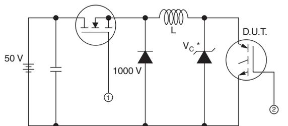
\* Driver same type as D.U.T.;  $V_C = 80\%$  of  $V_{ce(max)}$
