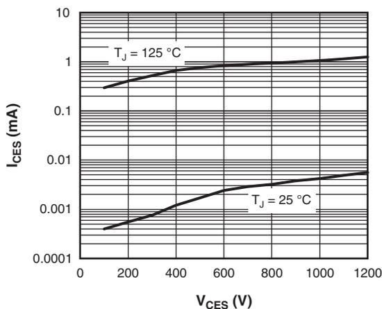
Fig. 6 - Typical IGBT Zero Gate Voltage Collector Current
