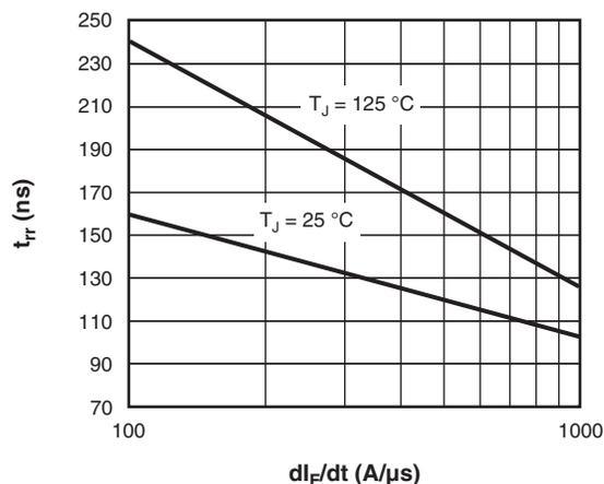
Fig. 13 - Typical  $t_{rr}$  diode vs.  $dI_F/dt$
