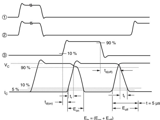
Fig. 18b - Switching Loss Waveforms Test Circuit
