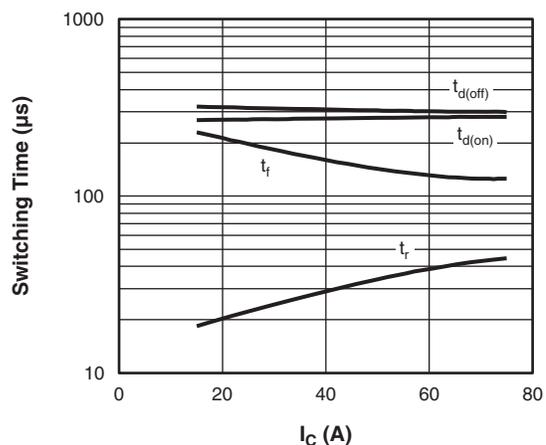
Fig. 10 - Typical IGBT Switching Time vs.  $I_C$
