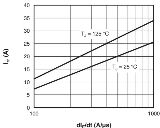
Fig. 14 - Typical  $I_{rr}$  diode vs.  $dI_F/dt$
