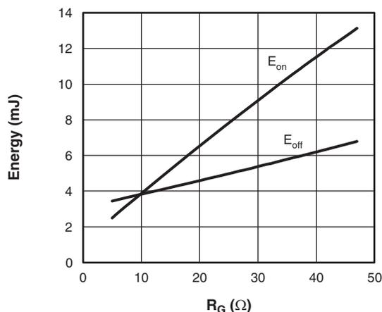
Fig. 11 - Typical IGBT Energy Loss vs.  $R_g$
