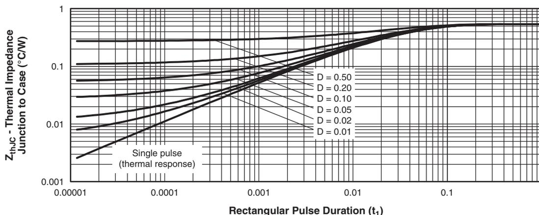
Fig. 16 - Maximum Thermal Impedance  $Z_{thJC}$  Characteristics (diode)
