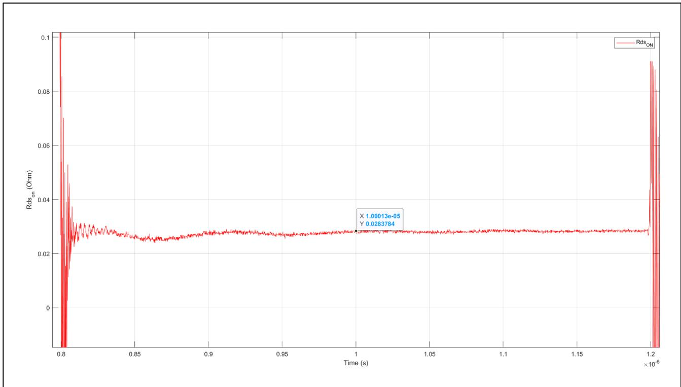
Figure: Red trace: 2<sup>nd</sup> Pulse  $R_{DSON}$  measurement of DUT. The device under test: GaN Systems 650V GaN GS6651B approximate  $R_{DSON} \approx 25m\Omega$ . Tell-i VON1k5Vm  $R_{DSON} \approx 28m\Omega$ .
