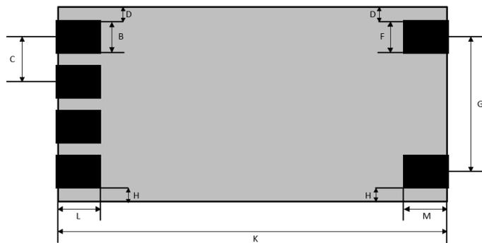
Figure. Bottom footprint with pad measurements for reflow-soldering
