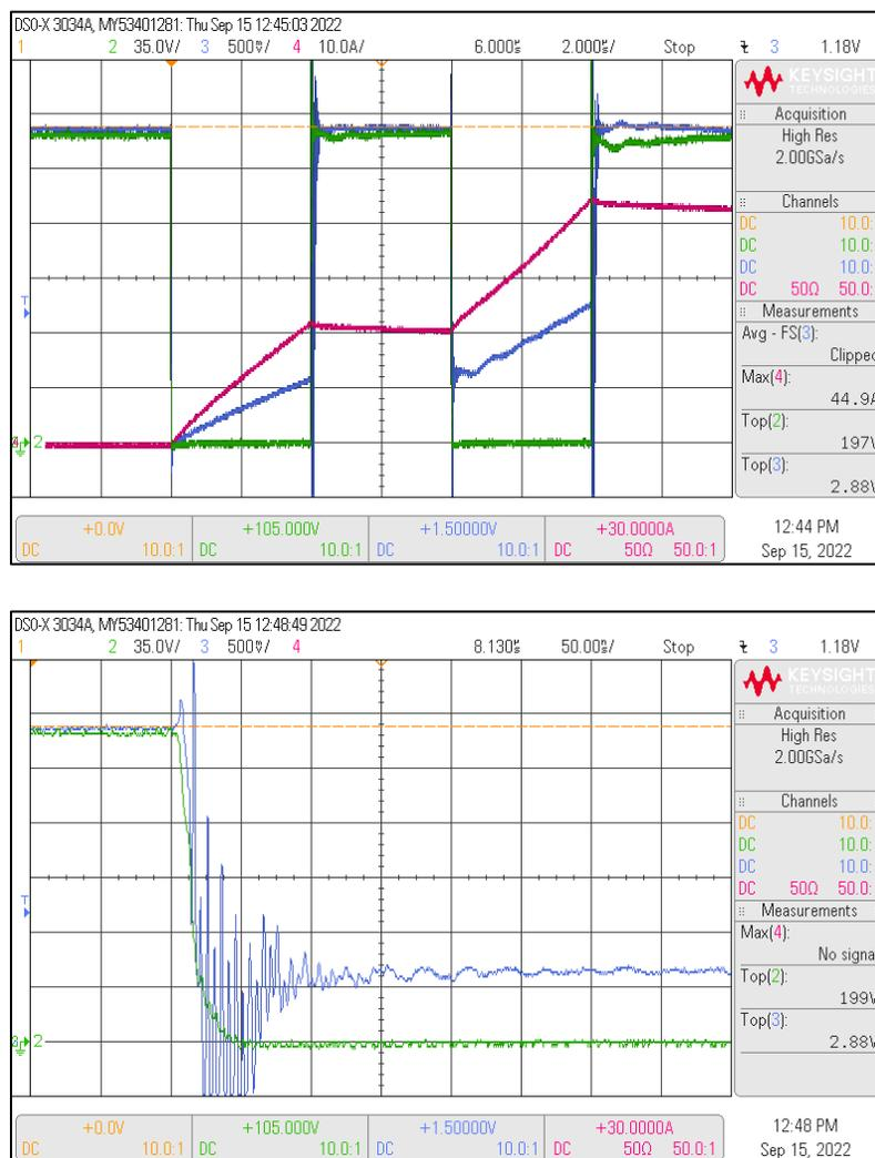
Figure: Double-pulse test: 200VDC, 45A. Green trace: Drain-Source Voltage. Blue trace: Tell-i VON1k5Vm output. Magenta trace: Inductor current. Tell-i VON1k5Vm settlement time: <50nsec. The device under test: GaN GS6651B.
