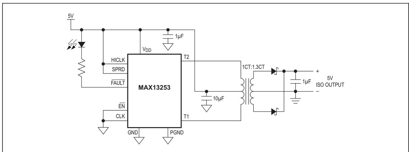
Figure 4. 5V to Isolated, Unregulated 6V Application Circuit
