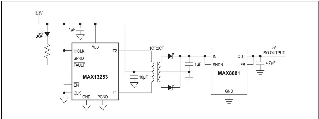
Figure 5. 3.3V to Isolated, Regulated 5V Application Circuit
