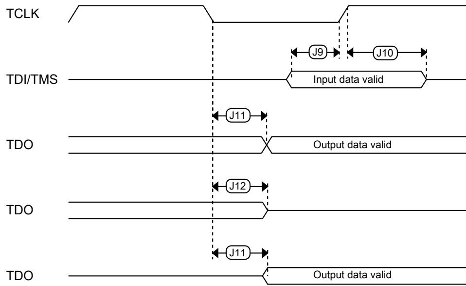
**Figure 9. Test Access Port timing**
