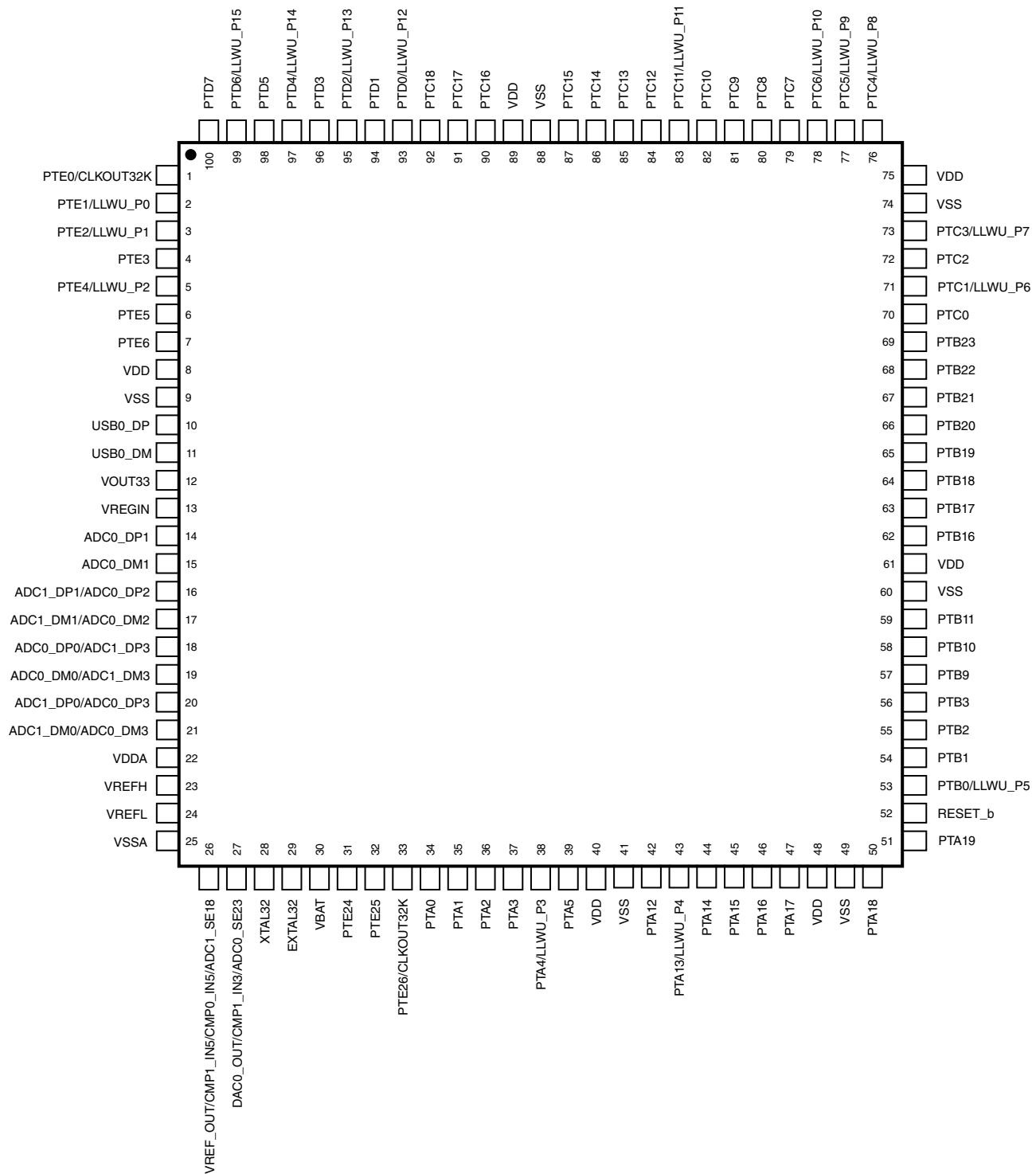
**Figure 35. K22F 100 LQFP pinout diagram (top view)**
