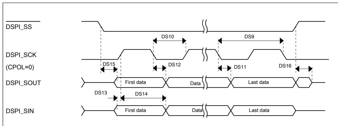
**Figure 24. DSPI classic SPI timing — slave mode**
