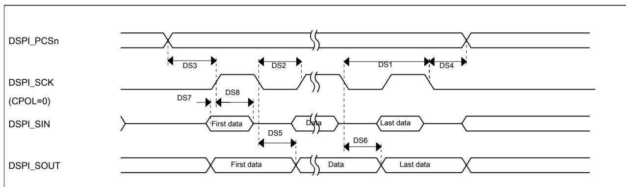
**Figure 23. DSPI classic SPI timing — master mode**
