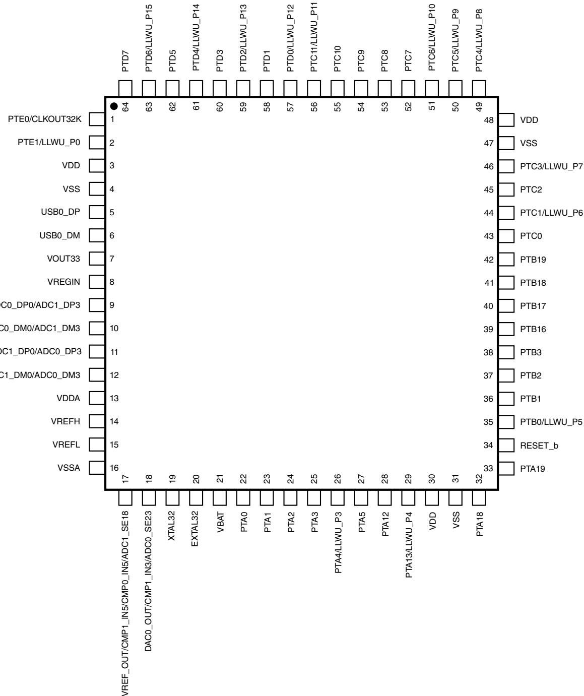
**Figure 32. K22F 64 LQFP pinout diagram (top view)**
