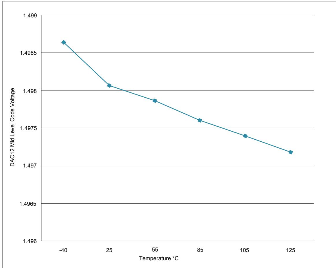
**Figure 20. Offset at half scale vs. temperature**
