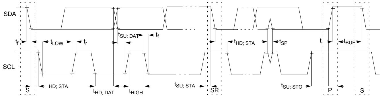
**Figure 25. Timing definition for devices on the I<sup>2</sup>C bus**
