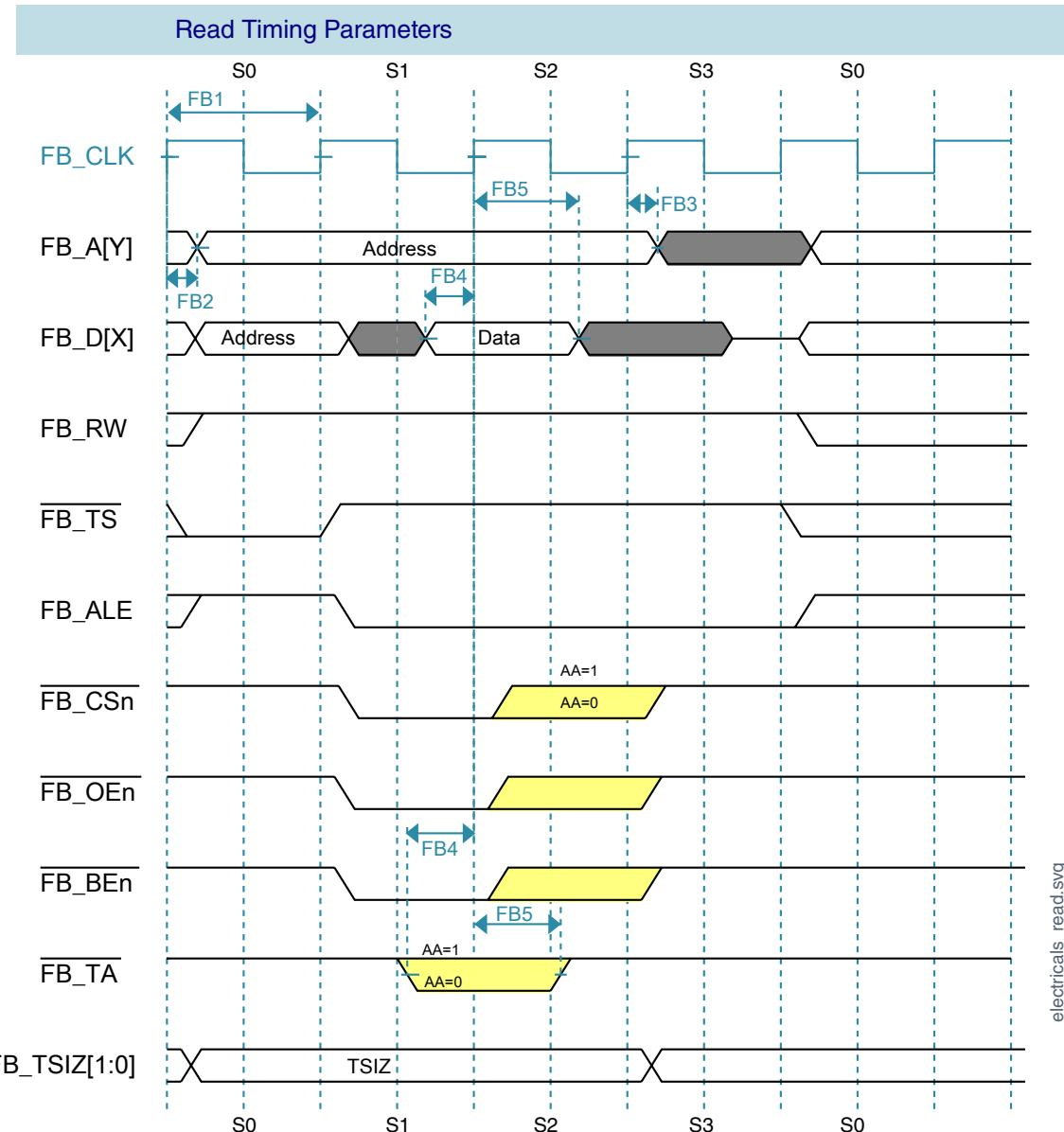
**Figure 12. FlexBus read timing diagram**
