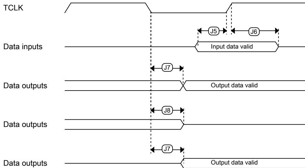
**Figure 8. Boundary scan (JTAG) timing**
