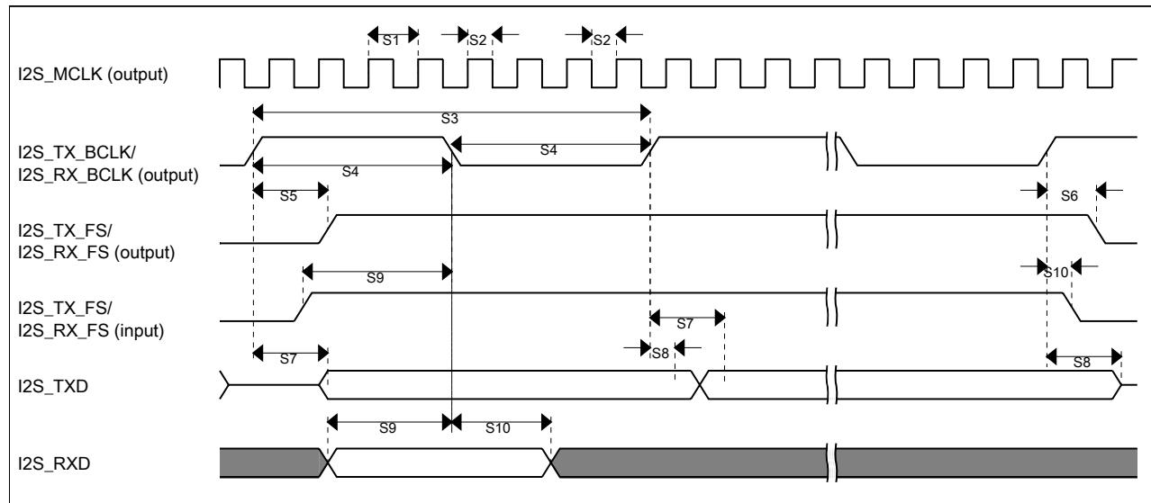
**Figure 28. I2S/SAI timing — master modes****Table 48. I2S/SAI slave mode timing in Normal Run, Wait and Stop modes (full voltage range)**
