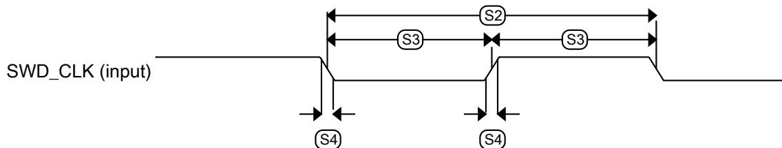
**Figure 5. Serial wire clock input timing**
