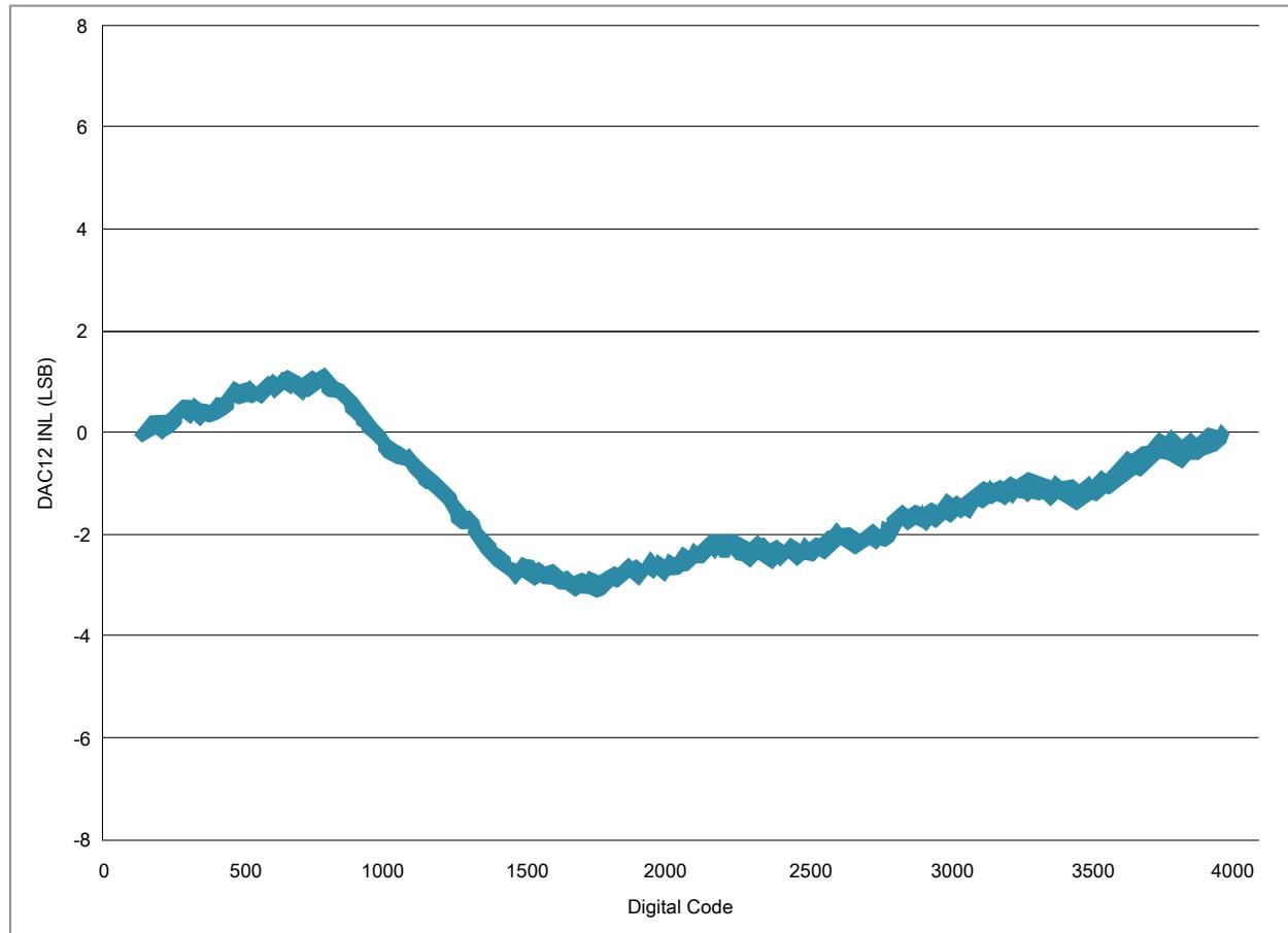
**Figure 19. Typical INL error vs. digital code**
