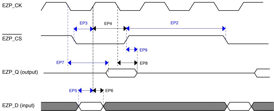
**Figure 11. EzPort Timing Diagram**
