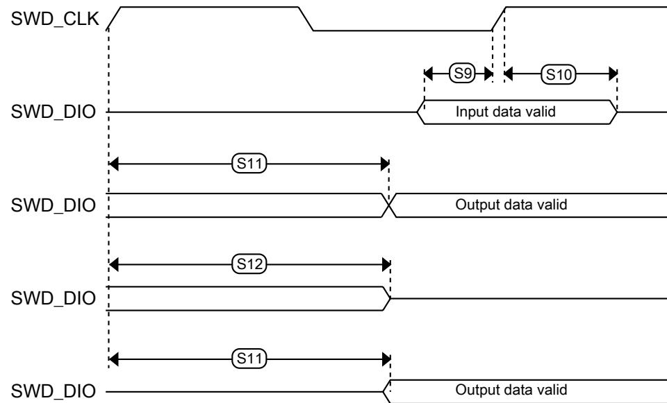
**Figure 6. Serial wire data timing**
