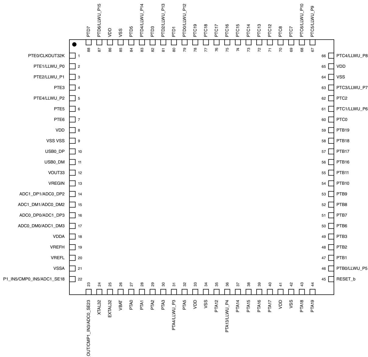
**Figure 34. K22F 88 QFN pinout diagram (transparent top view)**
