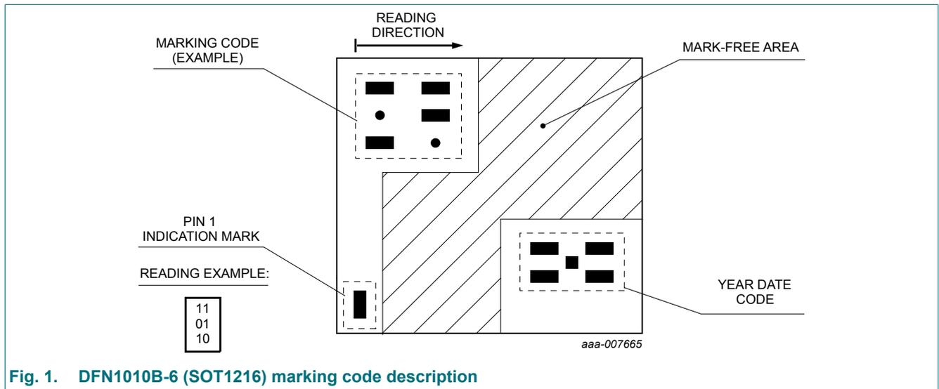
Fig. 1. DFN1010B-6 (SOT1216) marking code description
