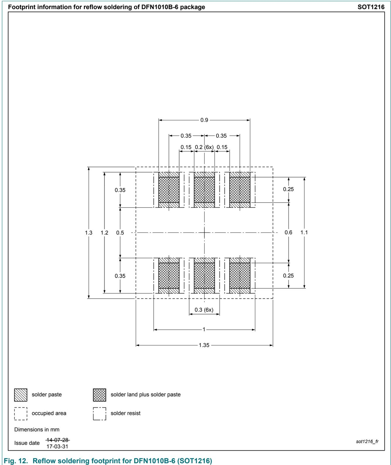
Fig. 12. Reflow soldering footprint for DFN1010B-6 (SOT1216)
