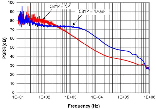
**Power Supply Ripple Rejection**
