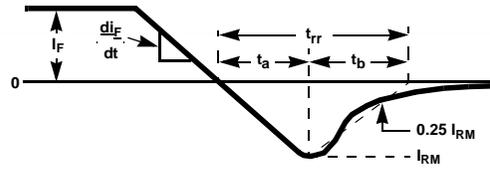
Figure 13.  $t_{rr}$  Waveforms and Definitions
