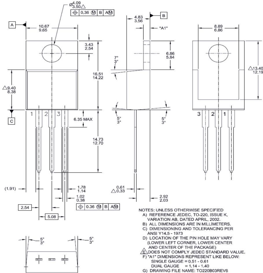
Figure 16. TO-220 3L - TO-220, MOLDED, 3LEAD, JEDEC VARIATION AB
