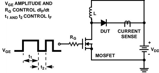
Figure 12.  $t_{rr}$  Test Circuit
