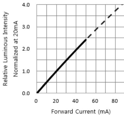
**Fig. 4 RELATIVE LUMINOUS INTENSITY VS. FORWARD CURRENT**
