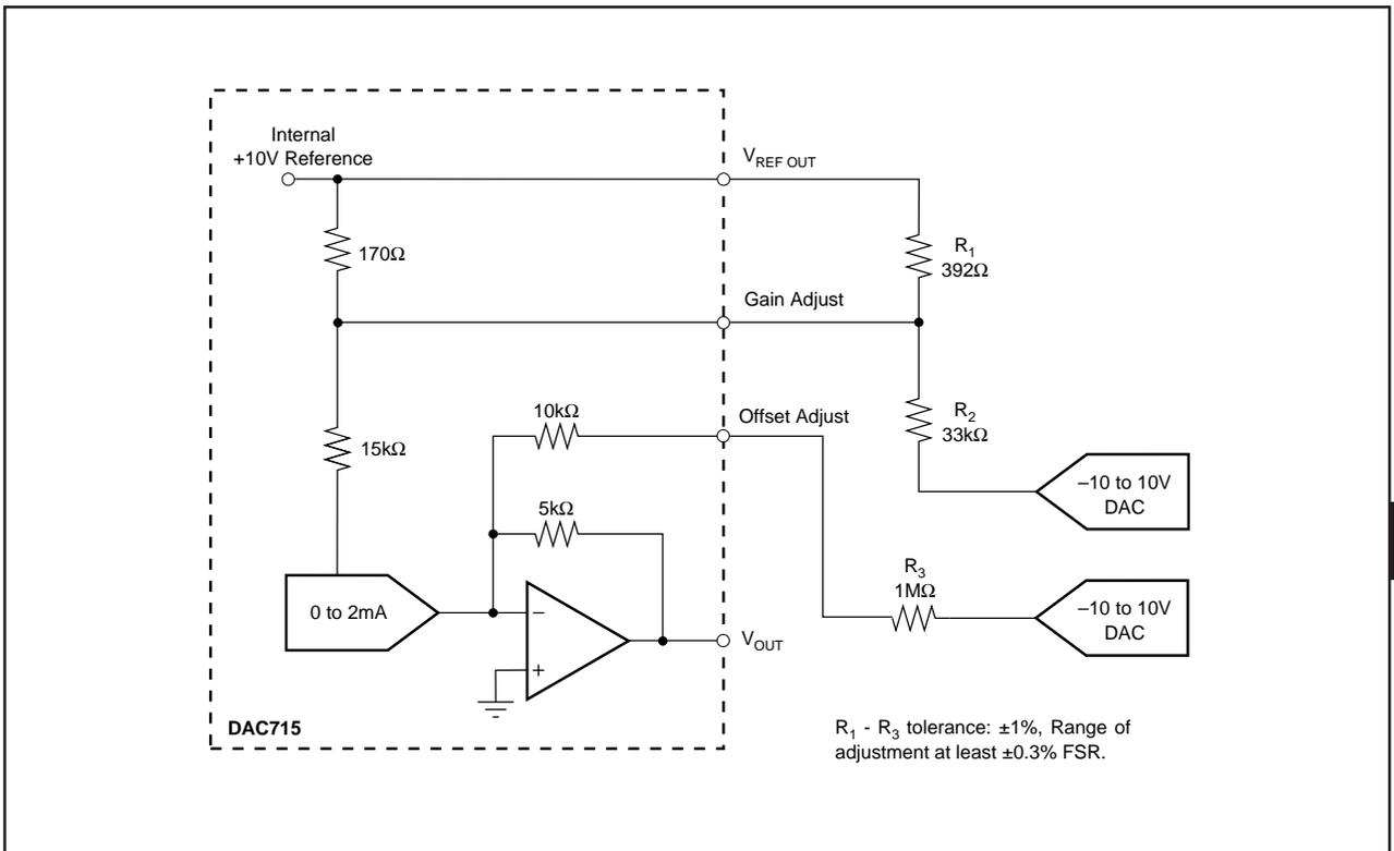
FIGURE 7. Gain and Offset Adjustment Using D/A Converters.
