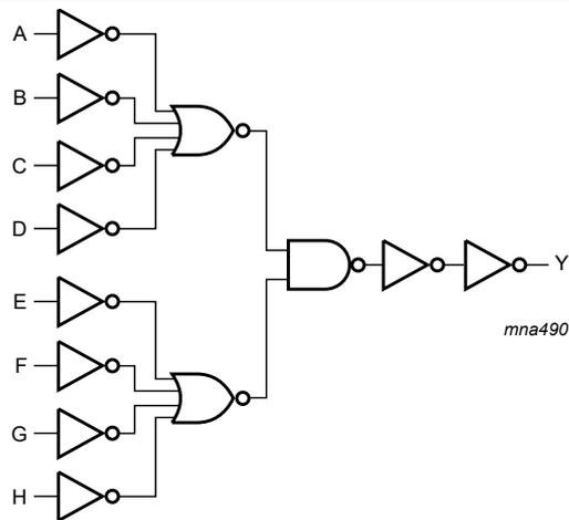
Fig. 3. Logic diagram
