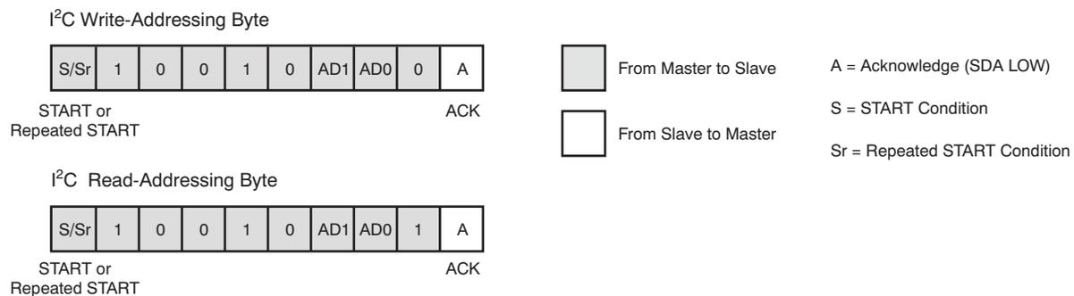
**Figure 34. I<sup>2</sup>C Bus Addressing (Slave Address Byte Format)**
