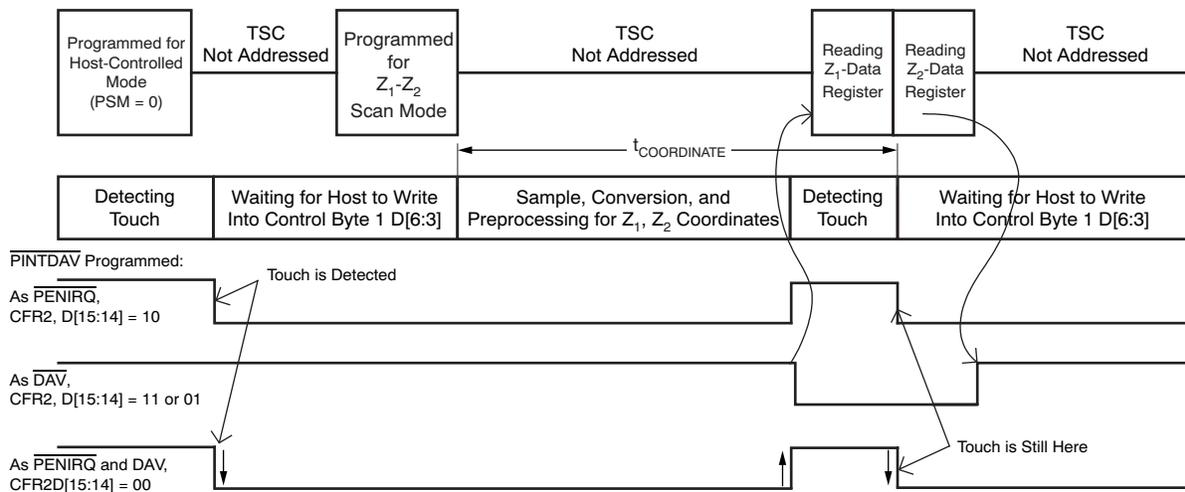
**Figure 44. Example of a Z<sub>1</sub> and Z<sub>2</sub> Coordinate Touch Screen Scan (with Panel Stabilization Time) using TSMODE 3**
