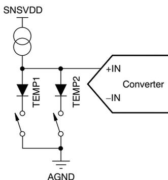
**Figure 27. Functional Block Diagram of Temperature Measurement Mode**
