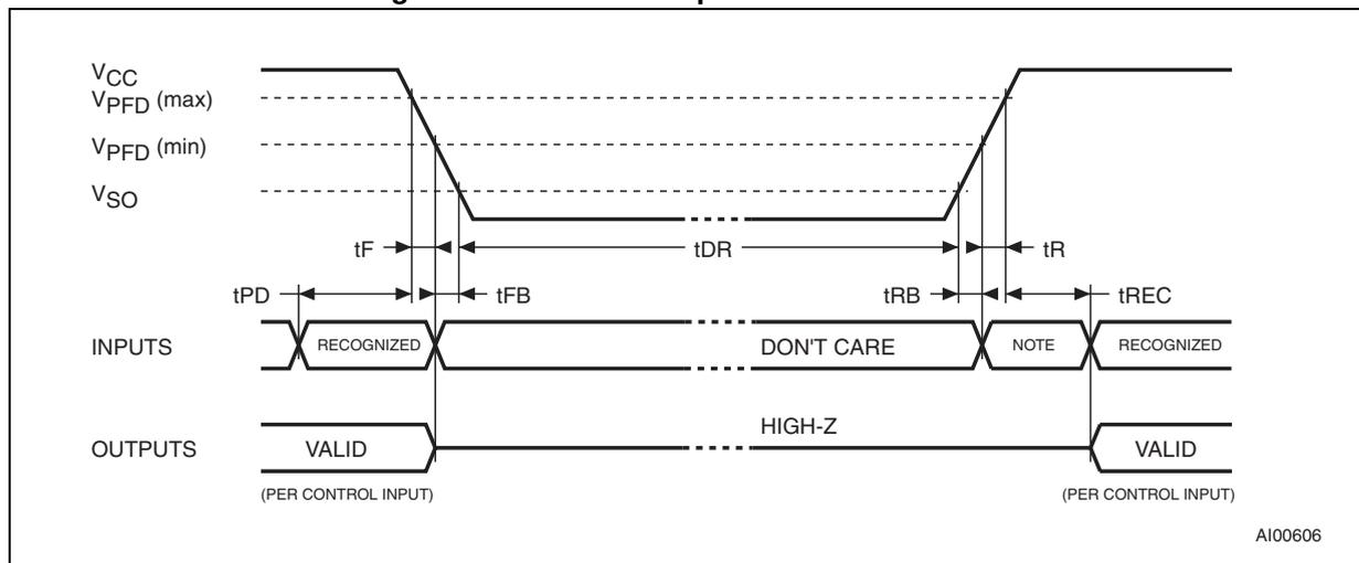
Note: Inputs may or may not be recognized at this time. Caution should be taken to keep  $\bar{E}$  high as  $V_{CC}$  rises past  $V_{PFD} (min)$ . Some systems may perform inadvertent WRITE cycles after  $V_{CC}$  rises above  $V_{PFD} (min)$  but before normal system operations begin. Even though a power on reset is being applied to the processor, a reset condition may not occur until after the system is running.
