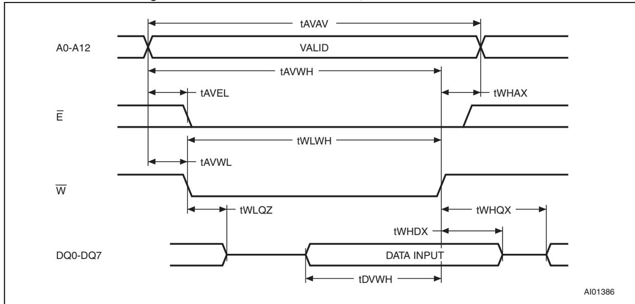
Figure 6. Chip enable controlled, WRITE AC waveforms
