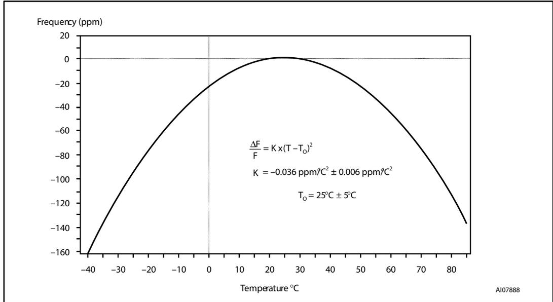
Figure 11: Clock calibration
