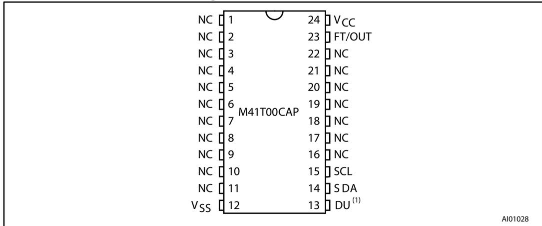
1. DU is "don't use". Do not connect. Must be allowed to float. Do not connect to  $V_{CC}$  or  $V_{SS}$ .
