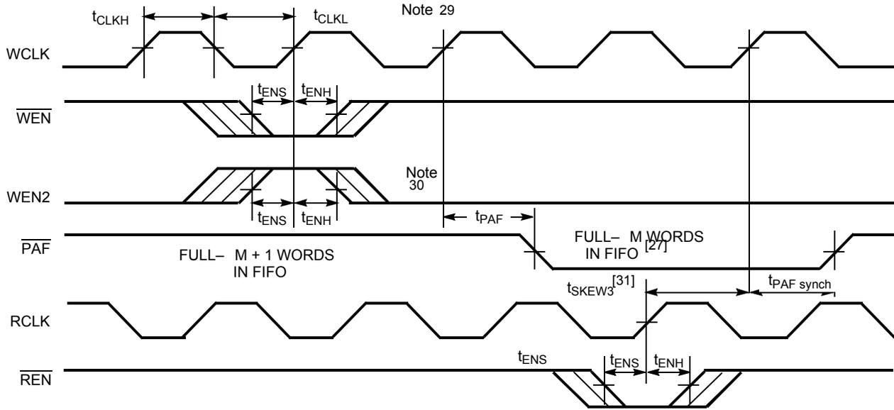
Figure 14. Write Programmable Registers
