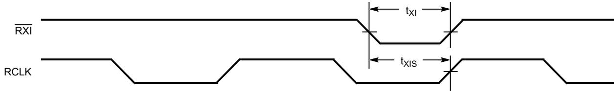
**Figure 20. Retransmit Timing**<sup>[34, 35, 36]</sup>
