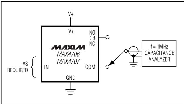
Figure 5. Channel Off/On-Capacitance
