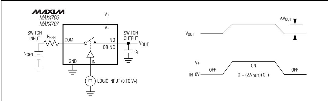
Figure 3. Charge Injection
