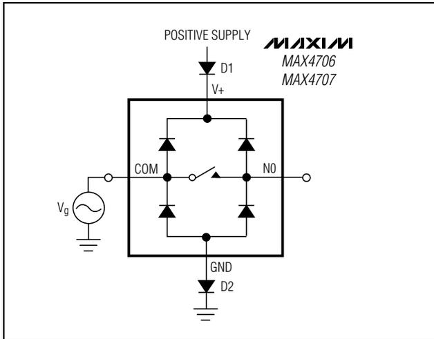
Figure 1. Overvoltage Protection Using Two External Blocking Diodes
