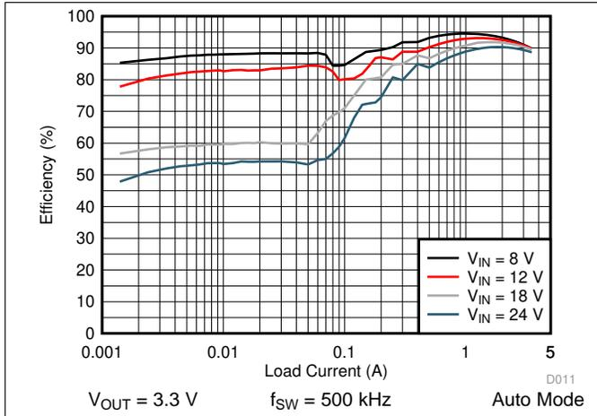
Figure 23. LM76003 Efficiency
