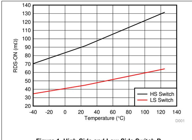
Figure 1. High-Side and Low-Side Switch R<sub>DS-ON</sub>
