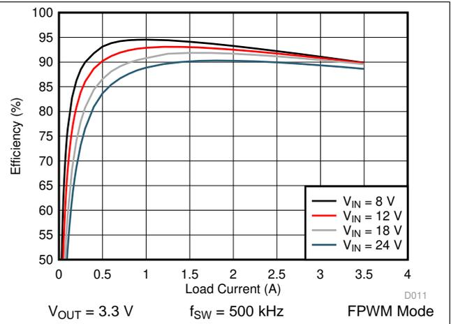
Figure 24. LM76003 Efficiency
