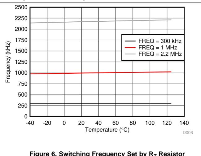
Figure 6. Switching Frequency Set by R<sub>T</sub> Resistor
