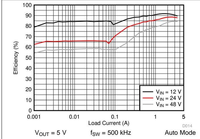
Figure 25. LM76003 Efficiency
