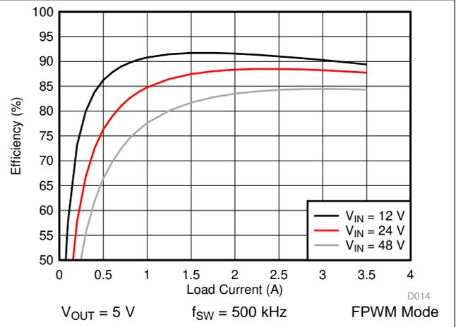
Figure 26. LM76003 Efficiency
