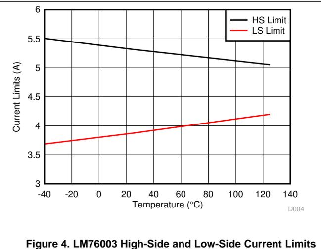
Figure 4. LM76003 High-Side and Low-Side Current Limits
