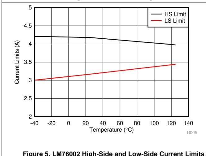
Figure 5. LM76002 High-Side and Low-Side Current Limits
