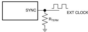
**Figure 18. Frequency Synchronization**
