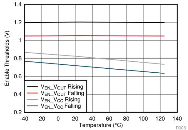
Figure 8. Enable Threshold
