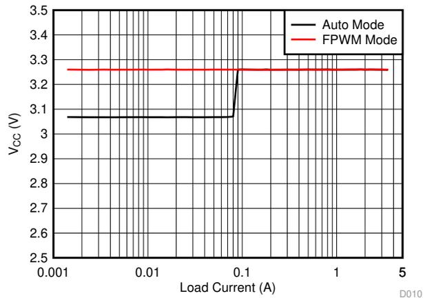
**Figure 13.  $V_{CC}$  Voltage Change With Mode Change**
