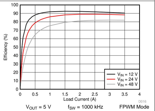
Figure 28. LM76003 Efficiency
