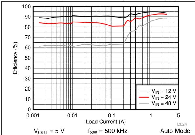
Figure 35. LM76002 Efficiency
