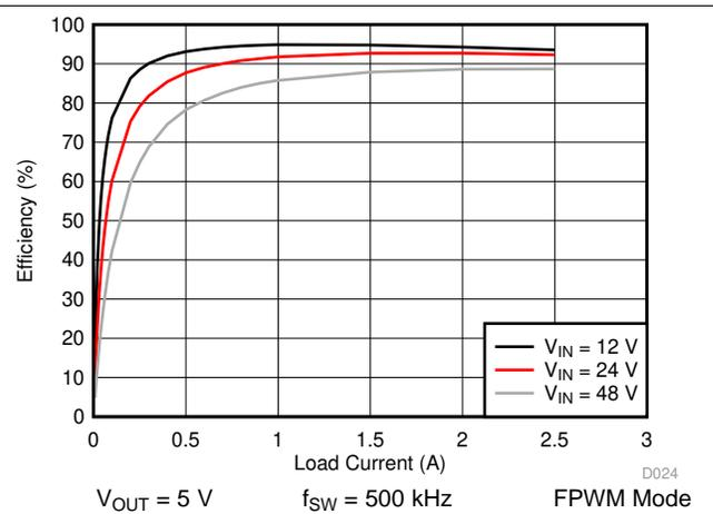
Figure 36. LM76002 Efficiency
