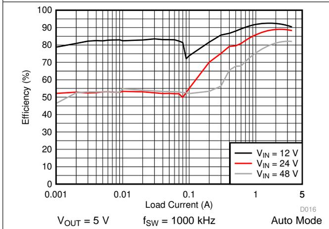
Figure 27. LM76003 Efficiency
