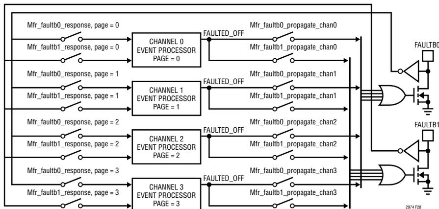
Figure 28. Channel Fault Management Block Diagram
