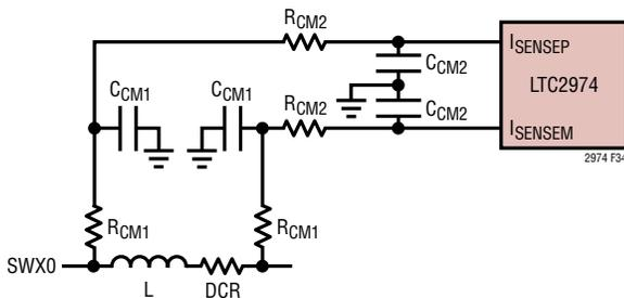
Figure 34. DCR Current Sensing Circuits
