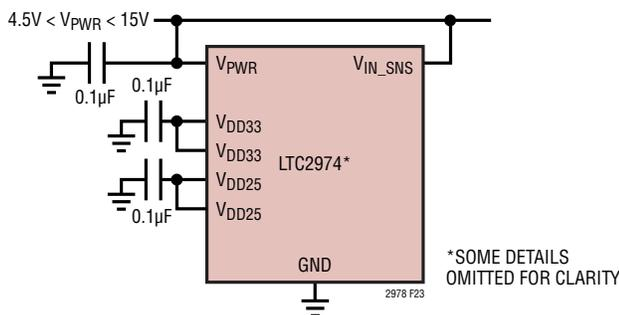
Figure 23. Powering LTC2974 Directly from an Intermediate Bus
