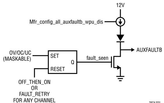
Figure 1. AUXFAULTB MUX
