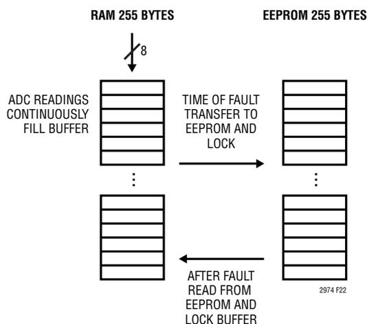
Figure 22. Fault Logging
