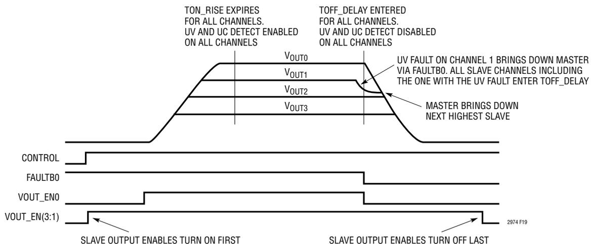
**Figure 19. Fault on Channel 1 Tracking All Supplies Down**
