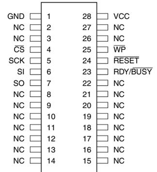
**Figure 2-4.** DataFlash Card<sup>(1)</sup> Top View through Package
