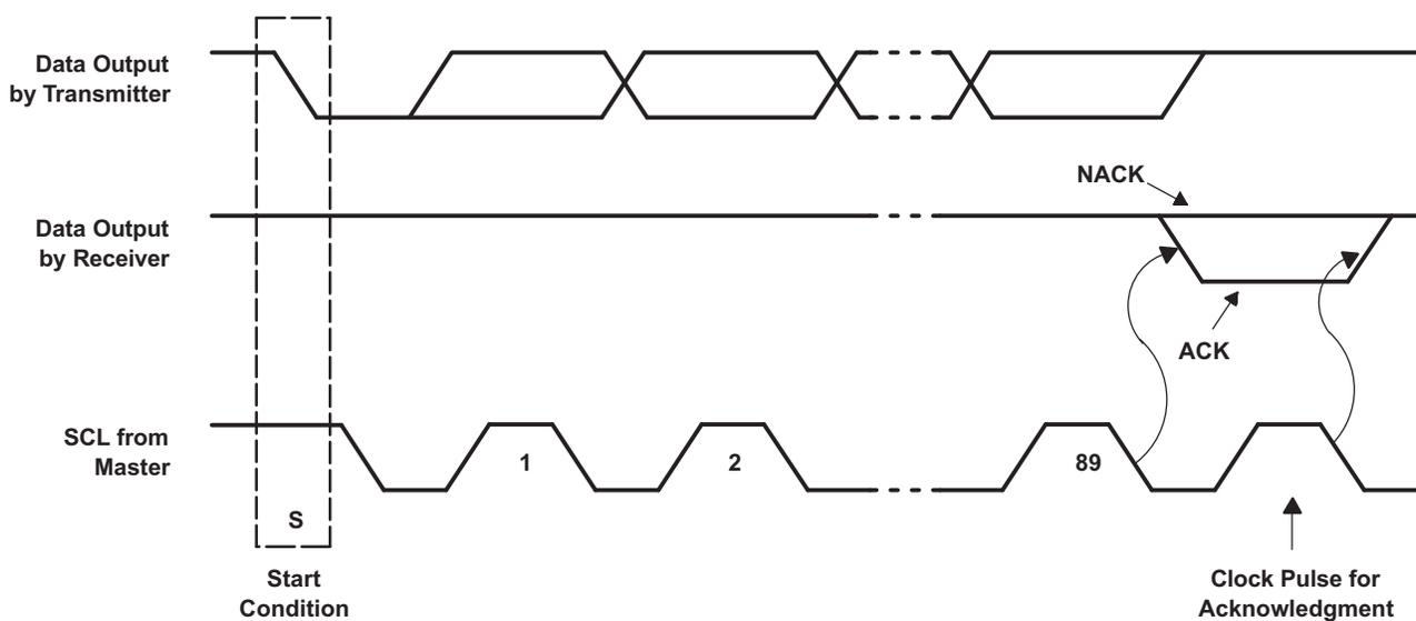
Figure 17. Acknowledgment on I<sup>2</sup>C Bus
