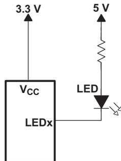
Figure 22. Device Supplied by a Lower Voltage
