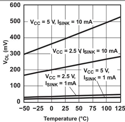
Figure 7. I/O Output Low Voltage vs Temperature
