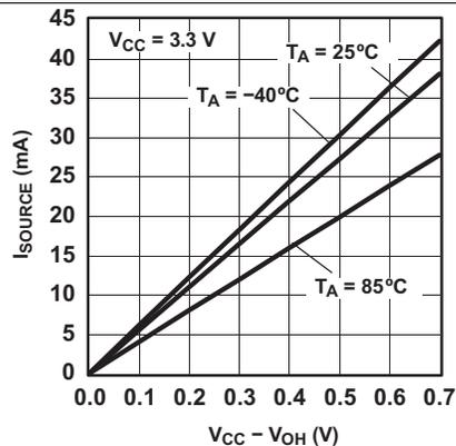
Figure 9. I/O Source Current vs Output High Voltage
