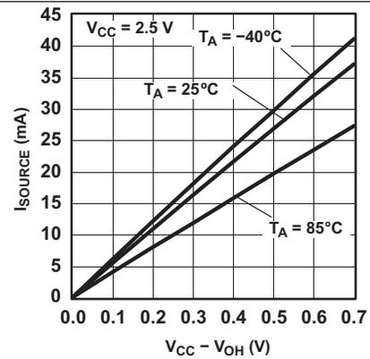
Figure 8. I/O Source Current vs Output High Voltage
