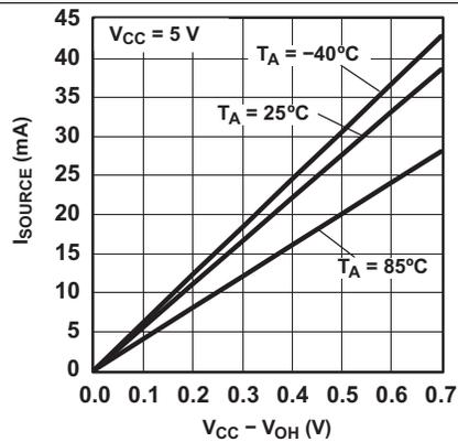
Figure 10. I/O Source Current vs Output High Voltage
