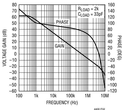
Figure 2. Measured Open-Loop Gain and Phase, PCTL < 80mV
