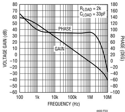
Figure 3. Measured Open-Loop Gain and Phase, PCTL > 160mV
