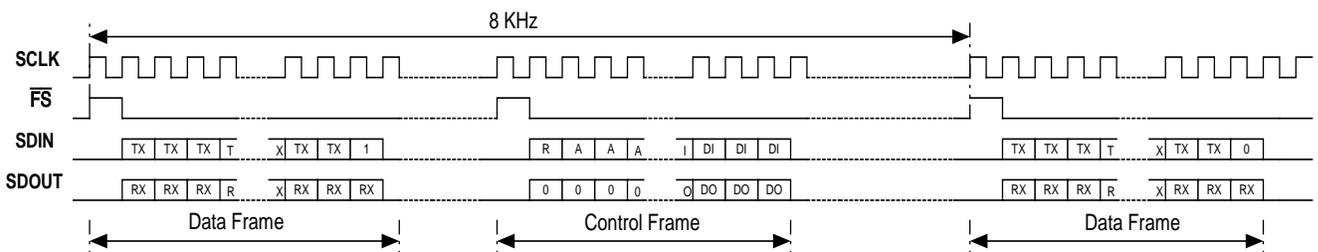
**Figure 18: Data and Control Frames Timing Diagram**
