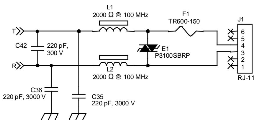
Figure 12: Suggested Over-voltage Protection and EMI Suppression Circuit
