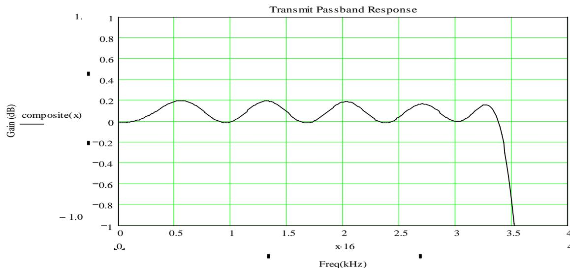
Figure 26: Pass-Band Response of the Transmit Path
