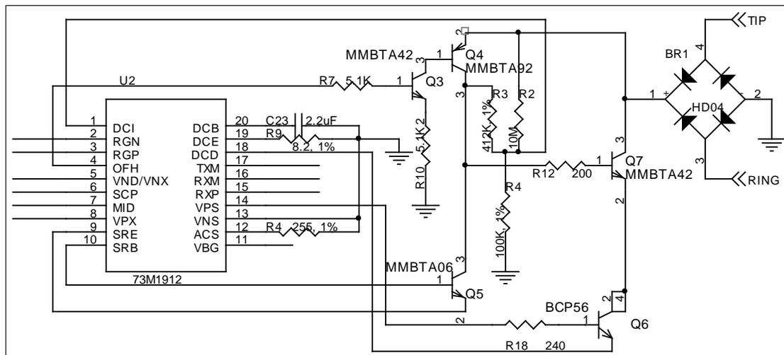
**Figure 30: Line-Side Device AC and DC Circuits**
