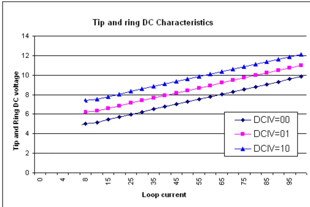
Figure 37: Off-Hook Tip and Ring DC Characteristics
