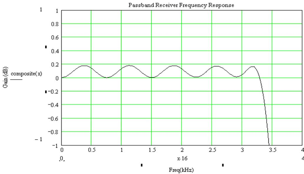
**Figure 29: Pass-band Response of the Overall Receive Path**
