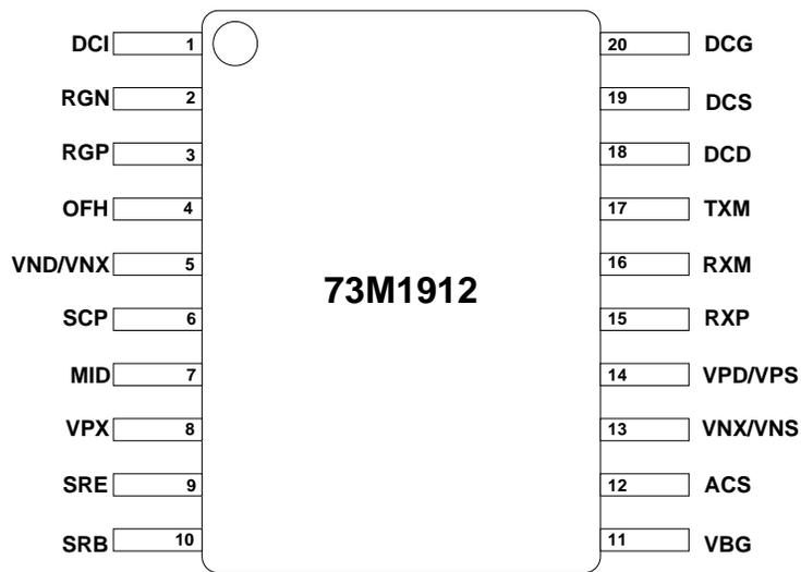
**Figure 3: 73M1912 20-Pin TSSOP Pinout**
