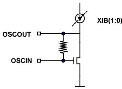
Figure 14: Crystal Oscillator with Configurable Load Current
