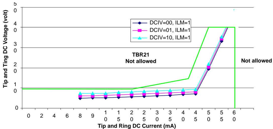
Figure 38: ES 203 021-2 DC Mask with Current Limit Enabled
