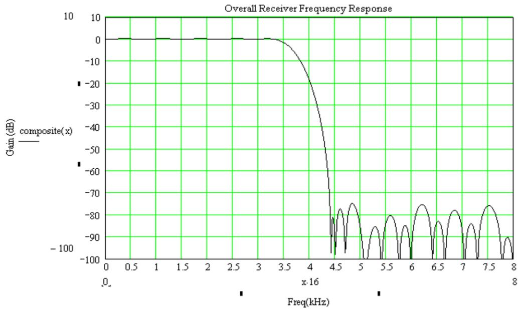
**Figure 28: Overall Frequency Response of the Receive Path**
