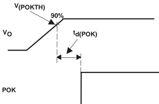
Figure 1. Power Okay Timing During Power Up
