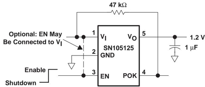
**Figure 9. Typical Application Schematic**
