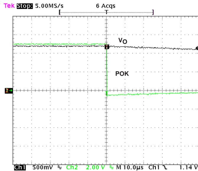
Figure 8. Power Okay Delay During Power Down Condition
