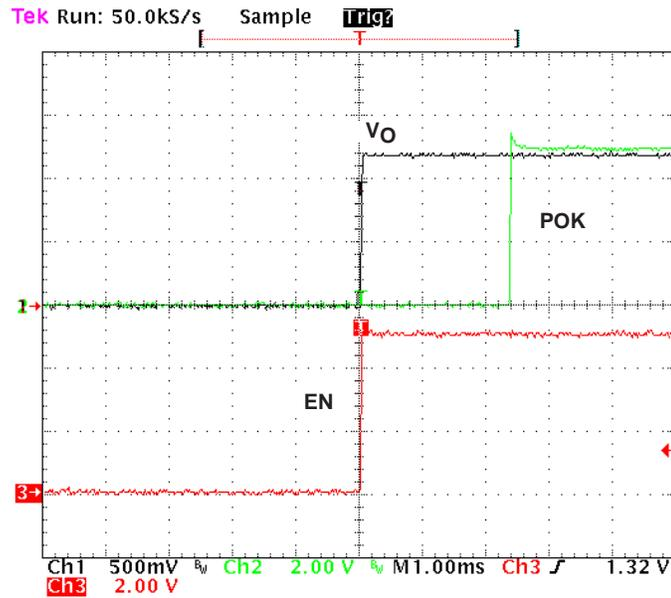
Figure 7. Power Okay Delay During Power Up Condition
