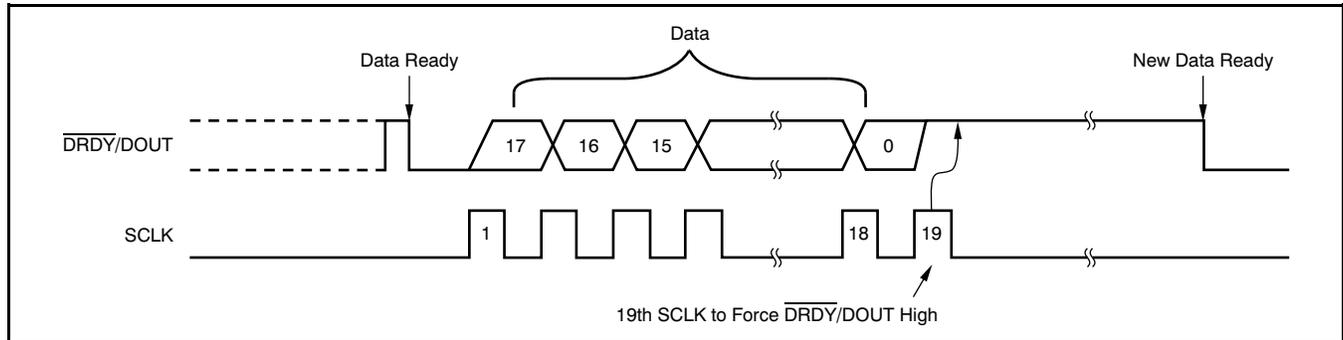
**Figure 7. Data Retrieval with  $\overline{\text{DRDY}}/\text{DOUT}$  Forced High Afterwards**
